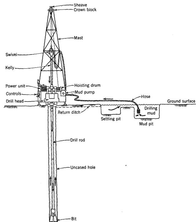
Figure 15. The principle of rotary drilling: arrows indicate direction of mud circulation. (after Davies & DeWiest)
