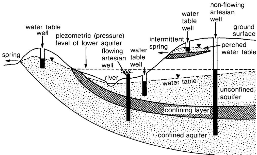
Figure 4. Disposition of groundwater and the borehole.
