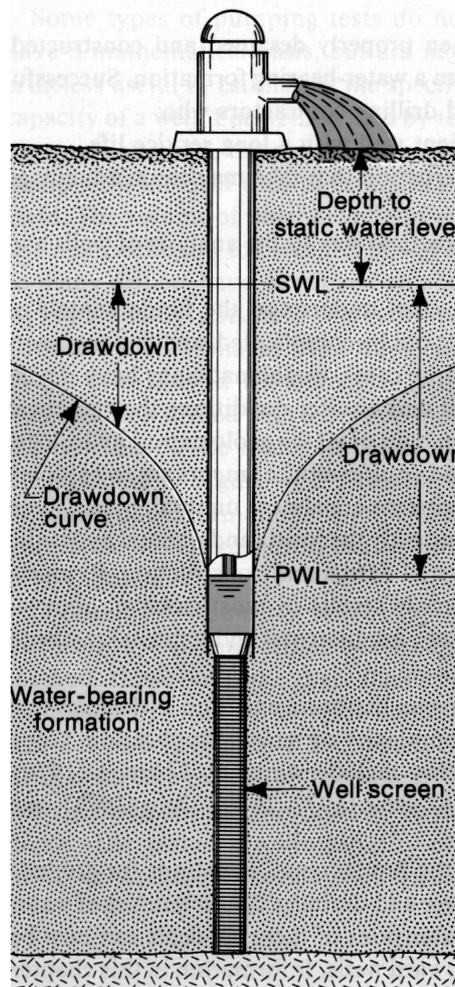
Figure 9. A high yielding borehole (motorised pump) shown here to emphasise significant drawdown, large screens and terminology (after Johnson)
