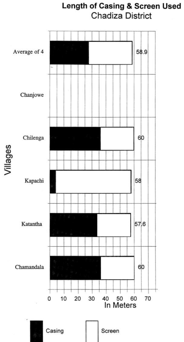
Figure 19. Borehole depths and casing/screens used.
