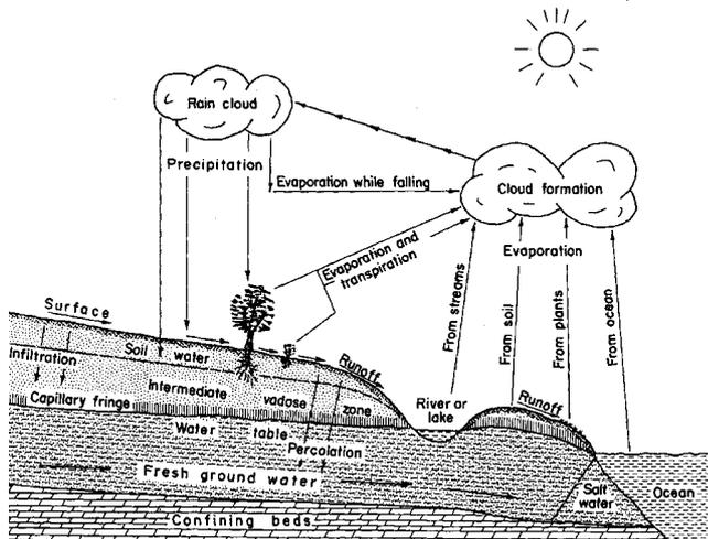
FIGURE 2. The Global water cycle or Hydrological cycle
