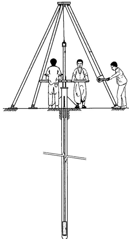
Figure 12. The auger method
