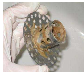
Fig. 8: Urine scale deposition on a waterless urinal's outlet sieve (old model) (source: L. Ulrich, December 2008)
