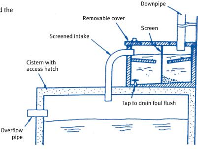
The run-off from a roof is directly proportional to the quantity of rainfall and the plan area of the roof. For every 1mm of rain a square metre of roof area will yield 1 litre of water, less evaporation, spillage losses and wind effects. The guttering and downpipes should be sized so as to be capable of carrying peak volume of run-off; in the tropics this can occur during high intensity storms of short duration.
