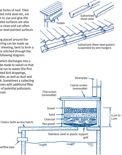
Alternatively, a foul flush box, which can be drained separately, may be fitted between the down-pipe and the storage tank, as shown in the following diagram:
