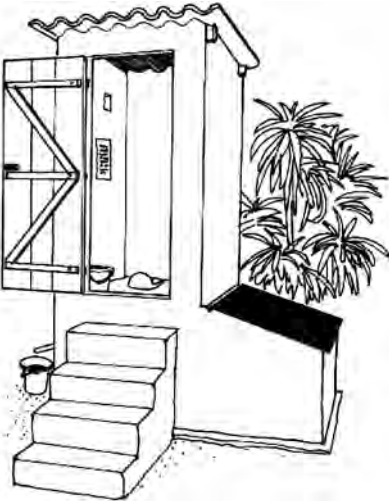
Figure 12: An eco-toilet with solar-heated processing chamber
