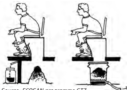
Figure 6: ECOSAN systems have two basic options for dealing with liquids: divert urine (left) or mix urine and faeces (right)
