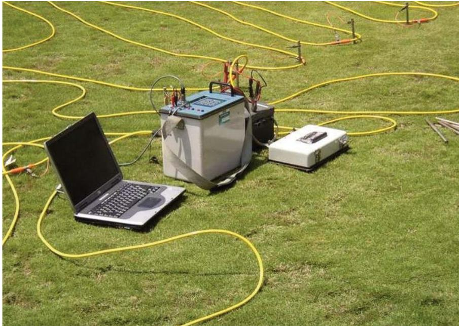
**Figure 4.5.2b.** A field layout for 2D resistivity imaging
