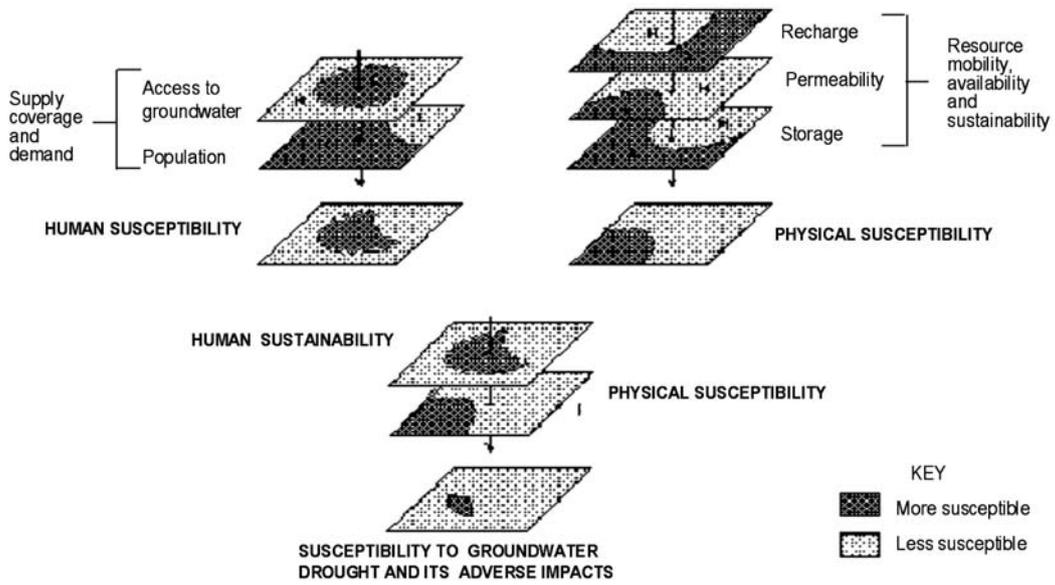
Figure 5.2.6. Example of drought susceptibility/vulnerability maps: Limpopo Province of South Africa (SADC, 2003b). Former 'homelands' are at risk due to a combination of skewed former ideology-based demographic coverage and difficult hydrogeological conditions.
