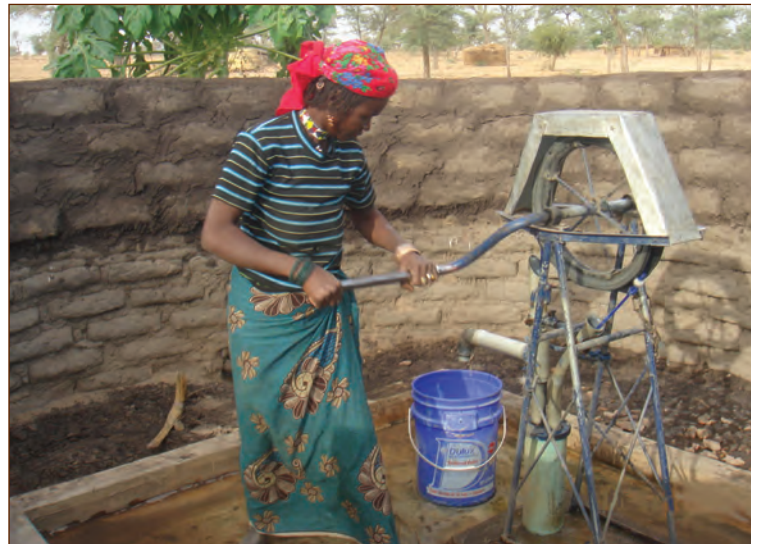
Rope Pump on Hand drilled Well
