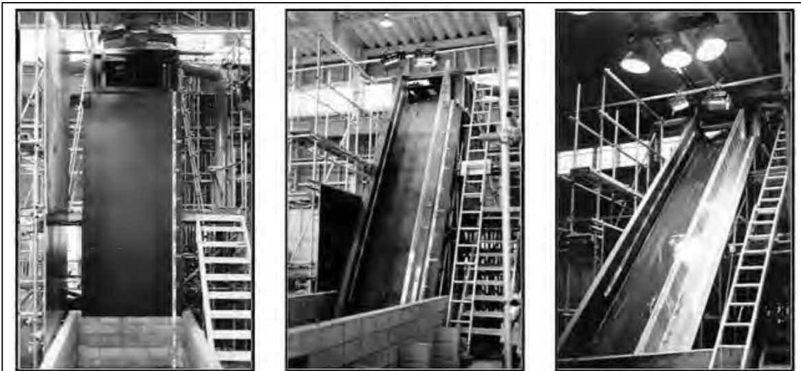
Figure 4 Experimental equipment. Those are 5m high, and the max flow rate is 0.1 m 3 /s.
