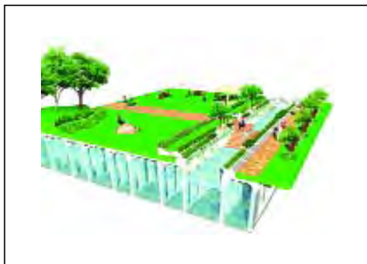
Fig. 17. Image of cistern ( park with water) for first-second fire-fighting phases
