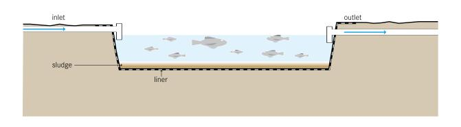
Fish can be grown in ponds that receive effluent or sludge where they can feed on algae and other organisms that grow in the nutrient-rich water. The fish, thereby, remove the nutrients from the wastewater and are eventually harvested for consumption.
