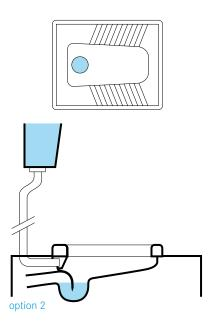
The cistern flush toilet is usually made of porcelain and is a mass-produced, factory-made User Interface. The flush toilet consists of a water tank that supplies the water for flushing the excreta and a bowl into which the excreta are deposited.
