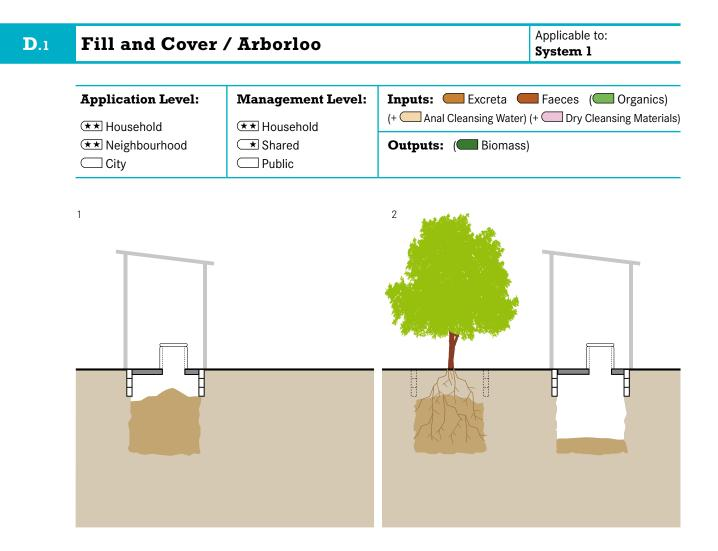
To decommission a pit, it can simply be filled with soil and covered. Although there is no benefit, the full pit poses no immediate health risk and the contents will degrade naturally over time. Alternatively, the Arborloo is a shallow pit that is filled with excreta and soil/ash and then covered with soil; a tree planted on top of the nutrient-rich pit will grow vigorously.
