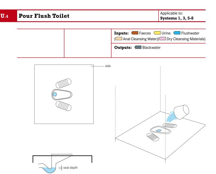
A pour flush toilet is like a regular Cistern Flush Toilet (U.5) except that the water is poured in by the user, instead of coming from the cistern above. When the water supply is not continuous, any Cistern Flush Toilet can become a pour flush toilet.
