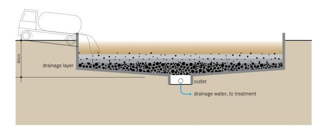
An unplanted drying bed is a simple, permeable bed that, when loaded with sludge, collects percolated leachate and allows the sludge to dry by evaporation. Approximately 50% to 80% of the sludge volume drains off as liquid or evaporates. The sludge, however, is not effectively stabilized or sanitized.
