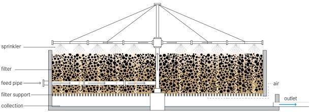
A trickling filter is a fixed-bed, biological reactor that operates under (mostly) aerobic conditions. Pre-settled wastewater is continuously 'trickled' or sprayed over the filter. As the water migrates through the pores of the filter, organics are degraded by the biofilm covering the filter material.
