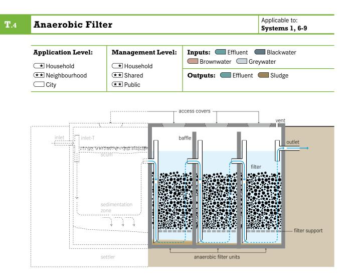
An anaerobic filter is a fixed-bed biological reactor with one or more filtration chambers in series. As wastewater flows through the filter, particles are trapped and organic matter is degraded by the active biomass that is attached to the surface of the filter material.
