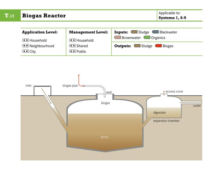
A biogas reactor or anaerobic digester is an anaerobic treatment technology that produces (a) a digested slurry (digestate) that can be used as a fertilizer and (b) biogas that can be used for energy. Biogas is a mix of methane, carbon dioxide and other trace gases which can be converted to heat, electricity or light.
