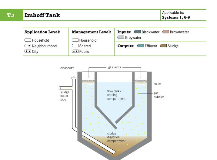
The Imhoff tank is a primary treatment technology for raw wastewater, designed for solid-liquid separation and digestion of the settled sludge. It consists of a V-shaped settling compartment above a tapering sludge digestion chamber with gas vents.
