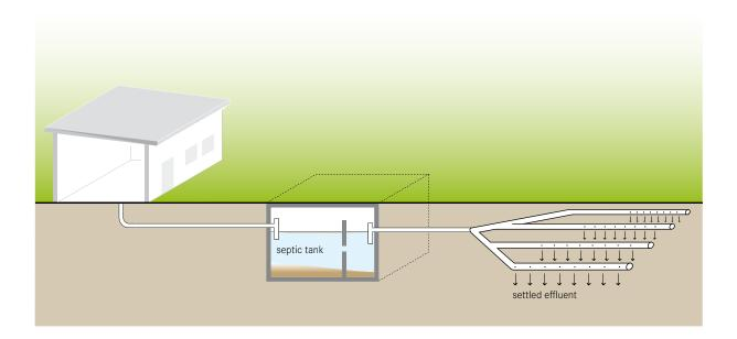
A leach field, or drainage field, is a network of perforated pipes that are laid in underground gravel-filled trenches to dissipate the effluent from a water-based Collection and Storage/Treatment or (Semi-) Centralized Treatment technology.
