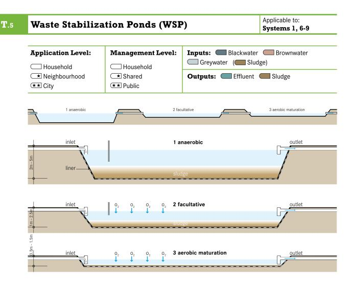
Waste Stabilization Ponds (WSPs) are large, manmade water bodies. The ponds can be used individually, or linked in a series for improved treatment. There are three types of ponds, (1) anaerobic, (2) facultative and (3) aerobic (maturation), each with different treatment and design characteristics.
