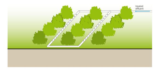
To reduce dependence on freshwater and maintain a constant source of water for irrigation throughout the year, wastewater of varying quality can be used in agriculture. However, only water that has had secondary treatment (i.e., physical and biological treatment) should be used to limit the risk of crop contamination and health risks to workers.
