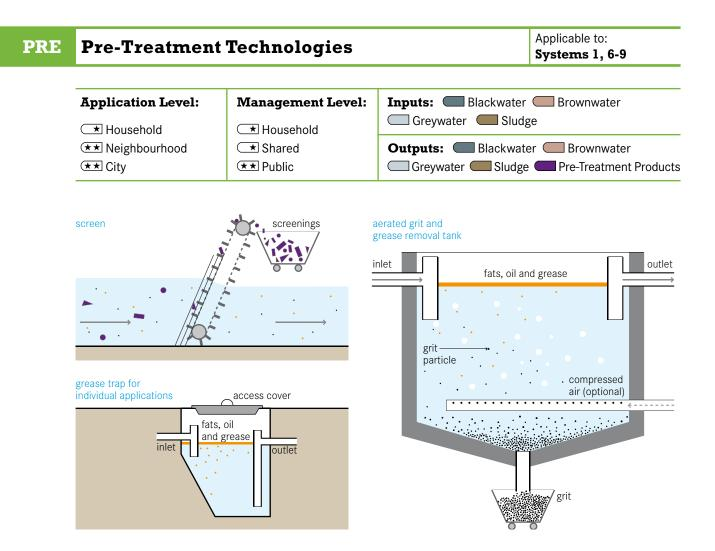
Pre-treatment is the preliminary removal of wastewater or sludge constituents, such as oil, grease, and various solids (e.g., sand, fibres and trash). Built before a Conveyance or Treatment technology, pre-treatment units can retard the accumulation of solids and minimize subsequent blockages. They can also help reduce abrasion of mechanical parts and extend the life of the sanitation infrastructure.
