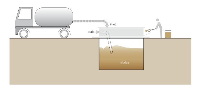
Transfer stations or underground holding tanks act as intermediate dumping points for faecal sludge when it cannot be easily transported to a (Semi-) Centralized Treatment facility. A vacuum truck is required to empty transfer stations when they are full.
