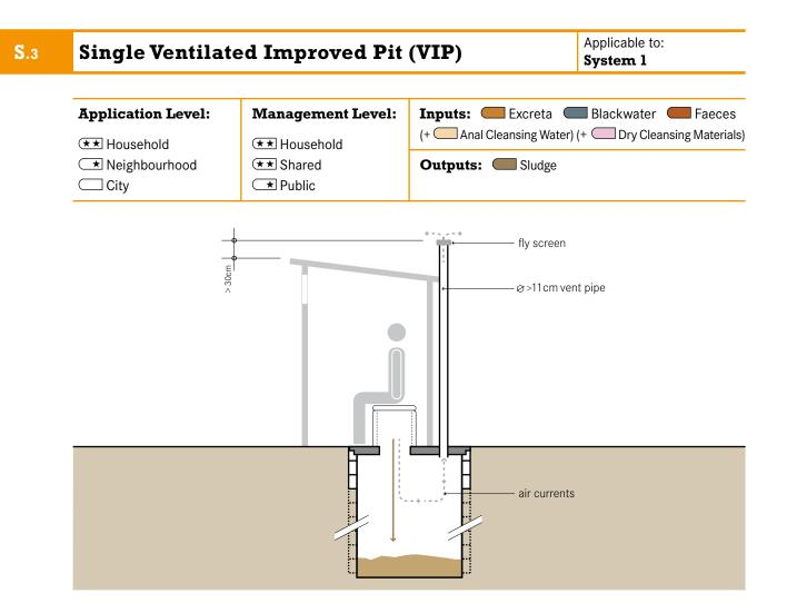
The single VIP is a ventilated improved pit. It is an improvement over the Single Pit (S.2) because continuous airflow through the ventilation pipe vents odours and acts as a trap for flies as they escape towards the light.
