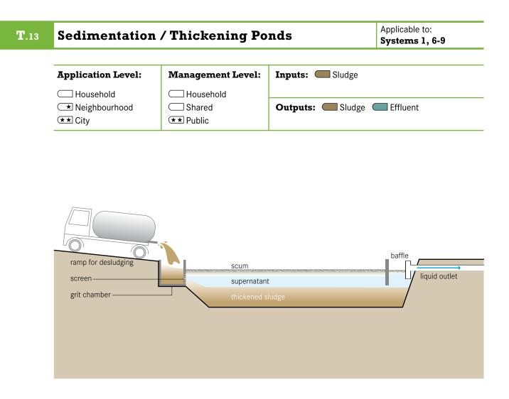
Sedimentation or thickening ponds are settling ponds that allow sludge to thicken and dewater. The effluent is removed and treated, while the thickened sludge can be further treated in a subsequent technology.
