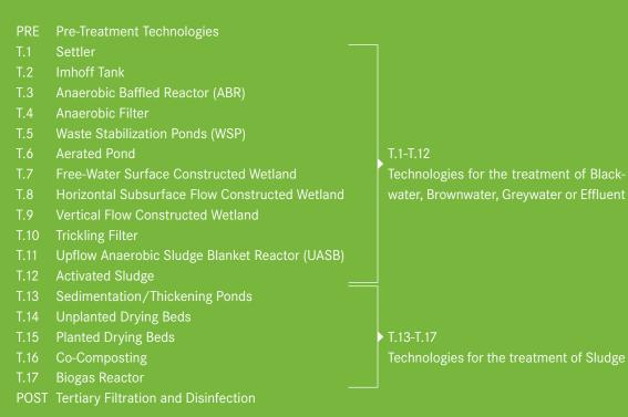
When designing a (Semi-) Centralized Treatment scheme, the engineer must create a meaningful combination of these technologies in order to achieve the desired overall treatment objective (e.g., a multiple-stage configuration for pre-treatment, primary treatment and secondary treatment).
