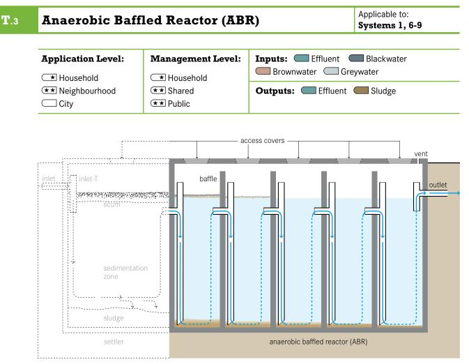
An anaerobic baffled reactor (ABR) is an improved Septic Tank (S.9) with a series of baffles under which the wastewater is forced to flow. The increased contact time with the active biomass (sludge) results in improved treatment.
