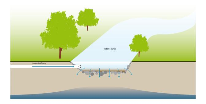
Treated effluent and/or stormwater can be directly discharged into receiving water bodies (such as rivers, lakes, etc.) or into the ground to recharge aquifers.
