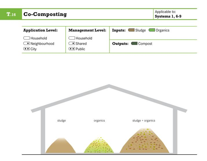
Co-composting is the controlled aerobic degradation of organics, using more than one feedstock (faecal sludge and organic solid waste). Faecal sludge has a high moisture and nitrogen content, while biodegradable solid waste is high in organic carbon and has good bulking properties (i.e., it allows air to flow and circulate). By combining the two, the benefits of each can be used to optimize the process and the product.
