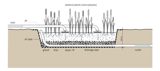
A vertical flow constructed wetland is a planted filter bed that is drained at the bottom. Wastewater is poured or dosed onto the surface from above using a mechanical dosing system. The water flows vertically down through the filter matrix to the bottom of the basin where it is collected in a drainage pipe. The important difference between a vertical and horizontal wetland is not simply the direction of the flow path, but rather the aerobic conditions.
