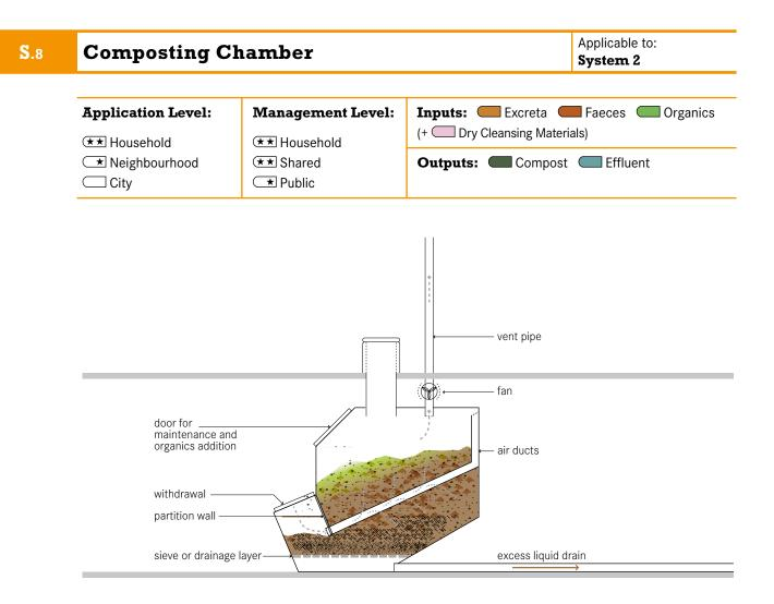
Composting refers to the process by which biodegradable components are biologically decomposed by microorganisms (mainly bacteria and fungi) under aerobic conditions. A composting chamber is designed to convert excreta and organics into compost. Compost is a stable, inoffensive product that can be safely handled and used as a soil conditioner.
