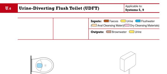
The urine-diverting flush toilet (UDFT) is similar in appearance to a Cistern Flush Toilet (U.5) except for the diversion in the bowl. The toilet bowl has two sections so that the urine can be separated from the faeces. Both sitting and squatting models exist.
