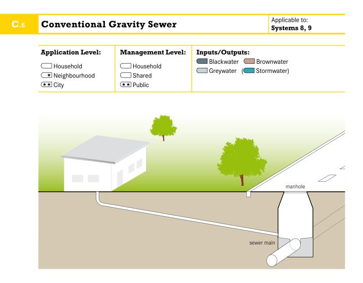
Conventional gravity sewers are large networks of underground pipes that convey blackwater, greywater and, in many cases, stormwater from individual households to a (Semi-) Centralized Treatment facility, using gravity (and pumps when necessary).
