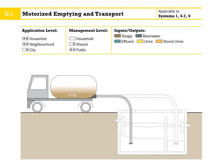
Motorized emptying and transport refers to a vehicle equipped with a motorized pump and a storage tank for emptying and transporting faecal sludge and urine. Humans are required to operate the pump and manoeuvre the hose, but sludge is not manually lifted or transported.
