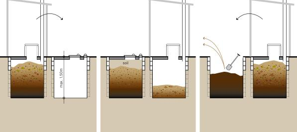
The Fossa Alterna is a short cycle alternating, waterless (dry) double pit technology. Compared to the Double VIP (S.4) which is just designed to collect, store and partially treat excreta, the Fossa Alterna is designed to make an earth-like product that can be used as a nutrient-rich soil conditioner. The Fossa Alterna is dug to a maximum depth of 1.5 m and requires a constant input of cover material (soil, ash, and/or leaves).
