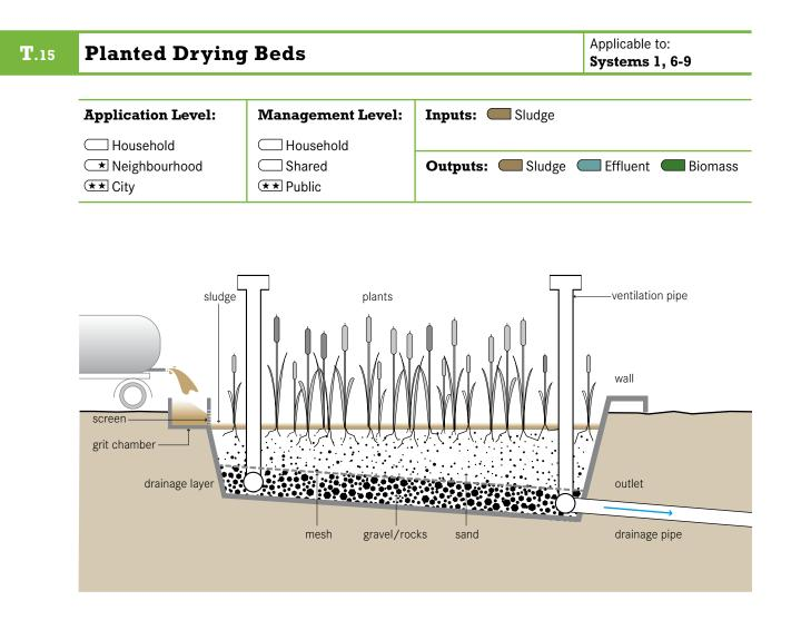
A planted drying bed is similar to an Unplanted Drying Bed (T.14), but has the added benefit of transpiration and enhanced sludge treatment due to the plants. The key improvement of the planted bed over the unplanted bed is that the filters do not need to be desludged after each feeding/drying cycle. Fresh sludge can be directly applied onto the previous layer; the plants and their root systems maintain the porosity of the filter.
