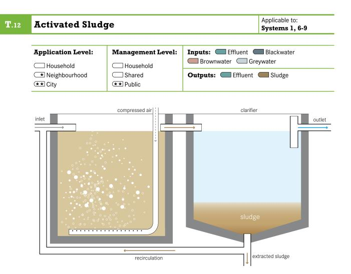
An activated sludge process refers to a multi-chamber reactor unit that makes use of highly concentrated microorganisms to degrade organics and remove nutrients from wastewater to produce a high-quality effluent. To maintain aerobic conditions and to keep the activated sludge suspended, a continuous and well-timed supply of oxygen is required.
