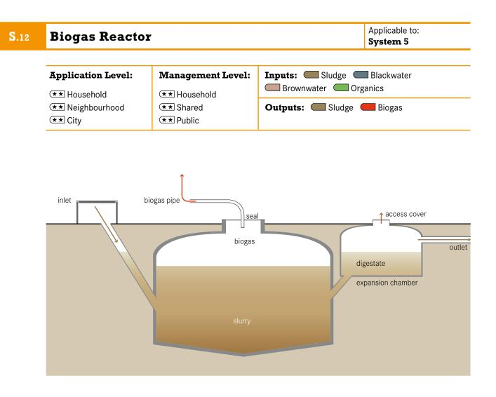
A biogas reactor or anaerobic digester is an anaerobic treatment technology that produces (a) a digested slurry (digestate) that can be used as a fertilizer and (b) biogas that can be used for energy. Biogas is a mix of methane, carbon dioxide and other trace gases which can be converted to heat, electricity or light.
