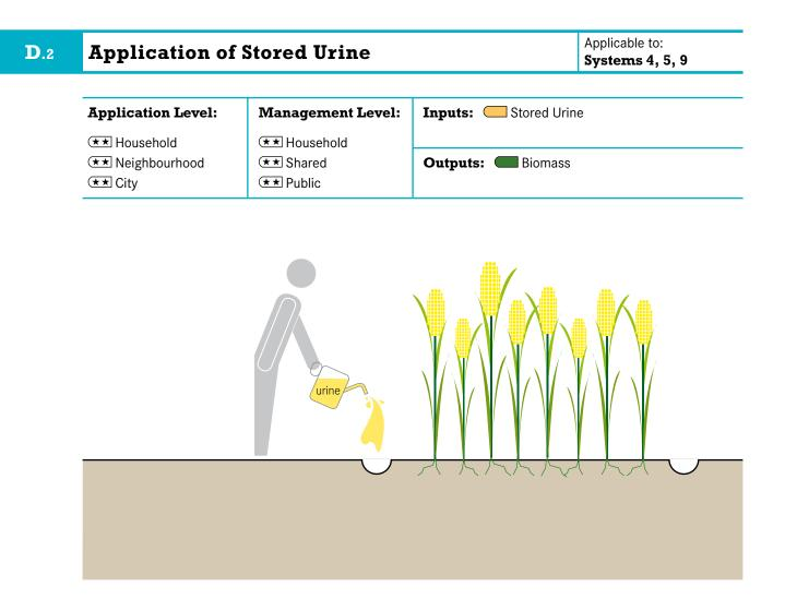
Stored urine is a concentrated source of nutrients that can be applied as a liquid fertilizer in agriculture and replace all or some commercial chemical fertilizers.
