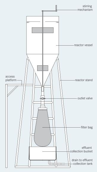
**Figure 7:** Schematic of a struvite reactor with stirring mechanism and filter bag
