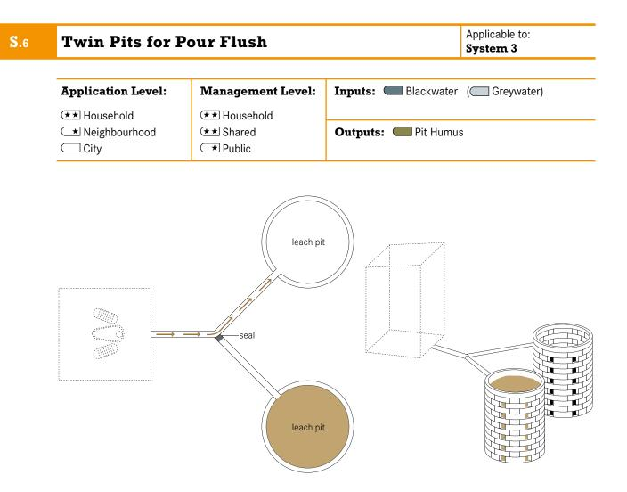
This technology consists of two alternating pits connected to a Pour Flush Toilet (U.4). The blackwater (and in some cases greywater) is collected in the pits and allowed to slowly infiltrate into the surrounding soil. Over time, the solids are sufficiently dewatered and can be manually removed with a shovel.
