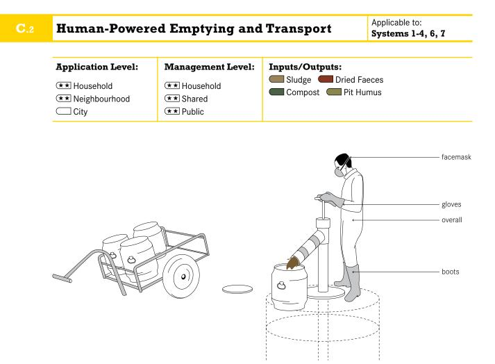
Human-powered emptying and transport refers to the different ways by which people can manually empty and/or transport sludge and solid products generated in onsite sanitation facilities.
