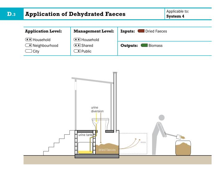
When faeces are stored in the absence of moisture (i.e., urine), they dehydrate into a crumbly, whitebeige, coarse, flaky material or powder. The moisture naturally present in the faeces evaporates and/or is absorbed by the drying material (e.g., ash, sawdust, lime) that is added to them. Dried faeces can be used as a soil conditioner.
