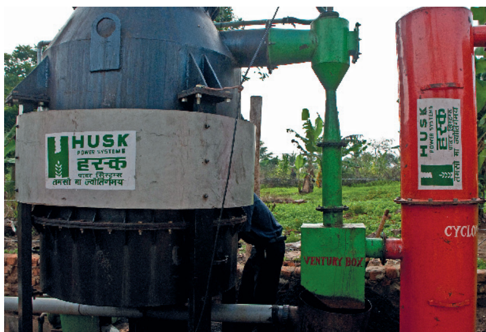
Figure 10.12 Iribigo gasification project utilising corn husks and sawdust, located in Muduma Sub-county, Mpigi District, Uganda (photo: Linda Strande).
