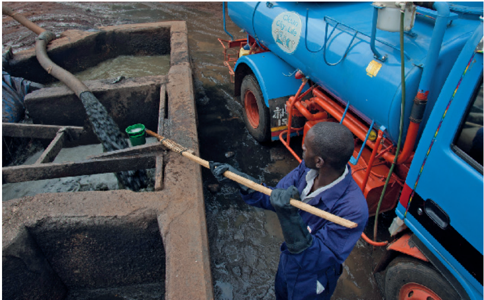
Figure 18.3 Implementation of the FAQ method (Faecal Sludge Quantification and Characterisation) in Kampala, Uganda (photo: Lars Schoebitz).
