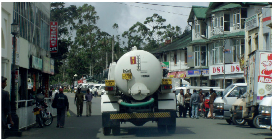
Figure 4.15 Sludge collection and transport vehicle navigating roads in the busy city of Manila, Philippines (photo: David M. Robbins).
