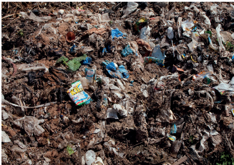
Figure 2.6 Municipal solid waste removed from faecal sludge with bar screens at treatment plant influent, Dakar, Senegal (photo: Linda Strande).
