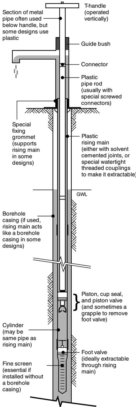
In most direct action handpump designs, the piston is raised and lowered by a 'T' bar handle, which is directly connected to an air-filled plastic pipe 'rod'. This rod floats in the water in the rising main, reducing the force needed on the upstroke. On the down-stroke, as more of the pipe rod enters the water in the rising main, it displaces an equal volume of water, so the pump delivers water on both the up-stroke and the down-stroke.
