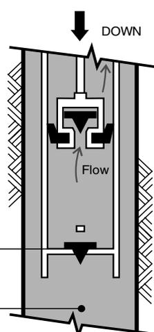
In most handpump cylinders a piston is alternately raised and lowered by a rod (or a string of rods joined together) which is connected to a handle, or sometimes to a flywheel and crank. These pumps are called **reciprocating handpumps**. The figure above illustrates how most cylinders work.
