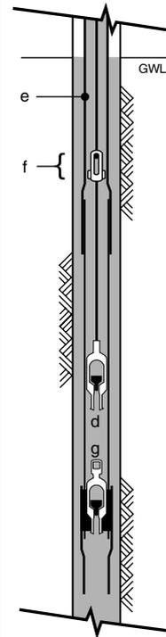
**Cylinder:** Recent deep-well pump designs have 'open top cylinders' (OTC). These allow the piston (d) to be pulled up through the rising main (e) which is of the same or, preferably, a slightly larger diameter than that of the cylinder. With these pumps, the piston can be pulled to the surface by pulling out the string of rods.
