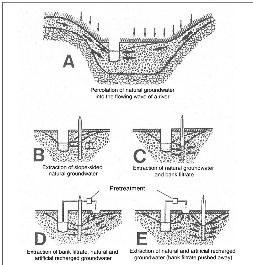
**Fig. 1.** Riverbank filtration and infiltration (artificial groundwater recharge).
