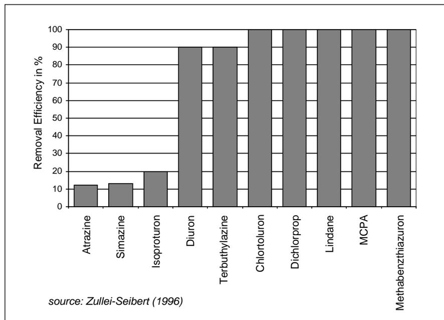
**Fig. 10.** Removal efficiency of artificial groundwater recharge for pesticide residues.
