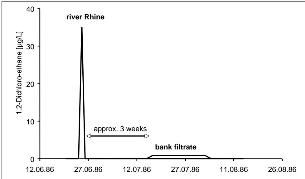
**Fig. 4.** Example of the protection against shock loads by bank filtration
