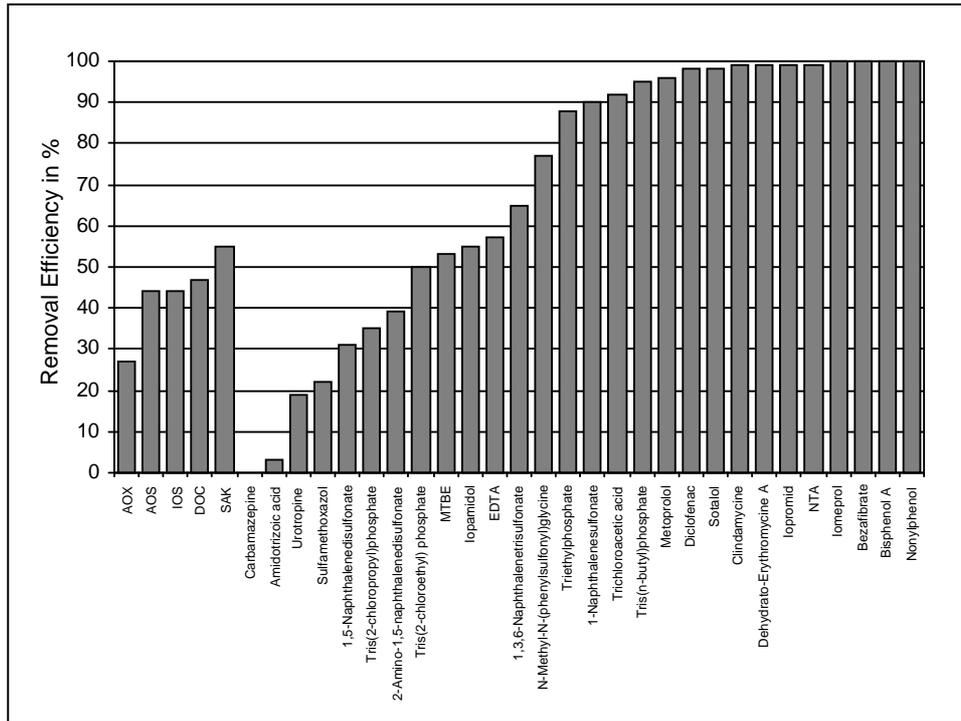
Fig. 11. Removal efficiency of riverbank filtration for micropollutants at the lower Rhine.
