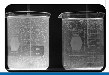
effects of different amounts of flocculation agents at different pH values to determine the right size floc for a particular plant. (The right size of floc depends upon the system's filter dimensions and other considerations.)
