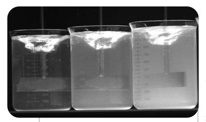
stirrers to match the conditions in the flocculator and allow them to operate for 30 minutes. Observe the floc formation periodically during the 30 minutes. At the end of the 30 minutes turn off the stirrers and allow settling. Most of the settling will be complete after one hour.
