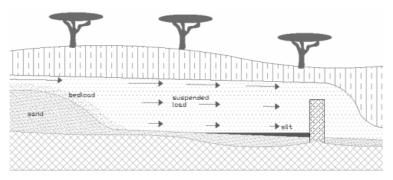
Figure 3: Schematic representation of the sedimentation process (Gijsbertsen, 2007)
