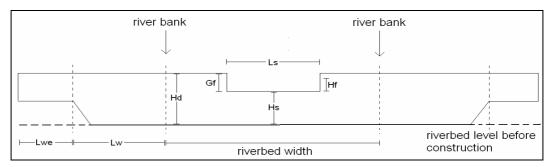
Figure 10: Cross section of a sand dam body and its dimensions.
