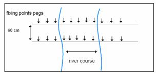
Figure 13: Example of setting a trench with pegs.
