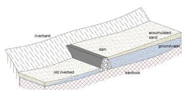
Figure 2: Schematic cross section of a typical sand storage dam (Borst & de Haas, 2006)
