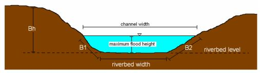
Figure 9: Cross section with maximum flood height to determine maximum discharge.
