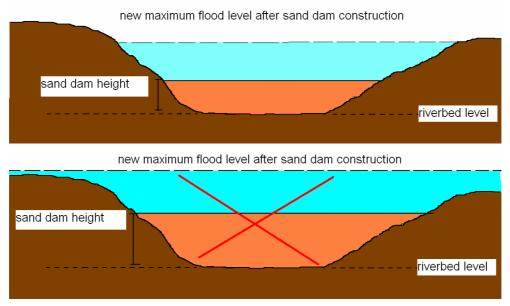
Figure 8: Examples of sand dam heights: do's and don't's.
