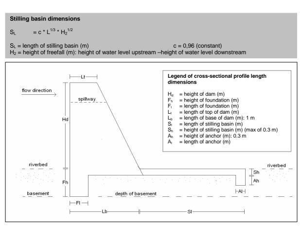
Figure 11: Cross sectional profile of a sand dam body and its dimensions.
