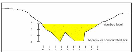
Figure 7: Example of cross profile and probing results.
