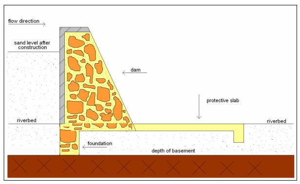
Figure 12: Cross sectional profile of a sand dam body.
