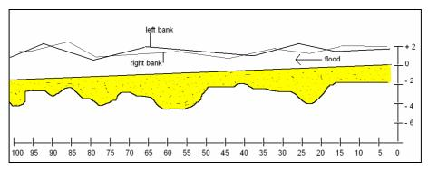
Figure 6: Example of a longitudinal profile of a river section.
