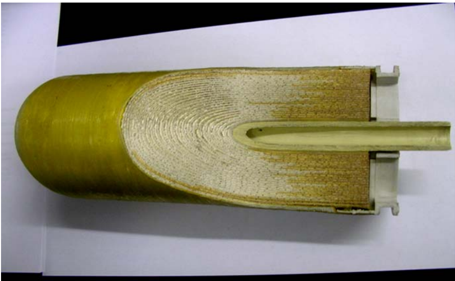
Fig. 5 Spiral-wound membrane part
