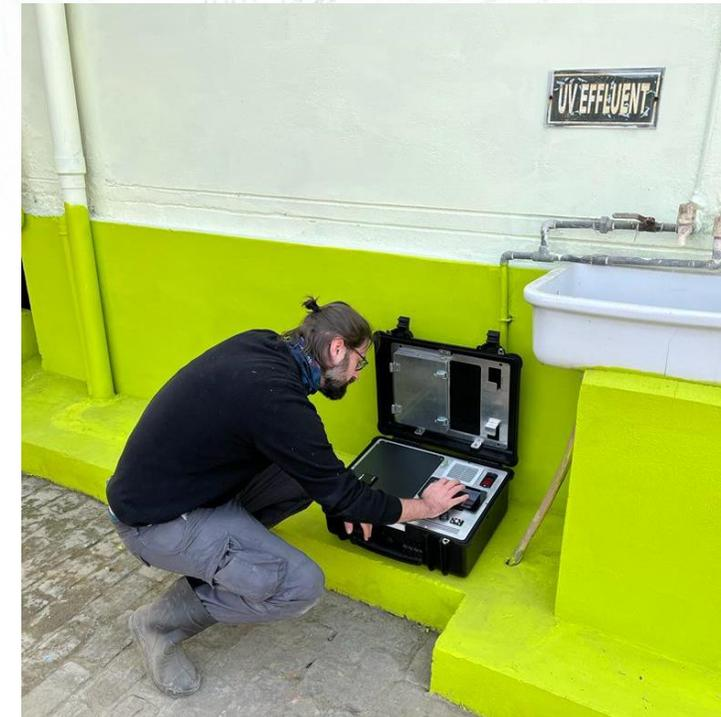
Sensor calibration in UV Effluent tap in Aligarh (India)
