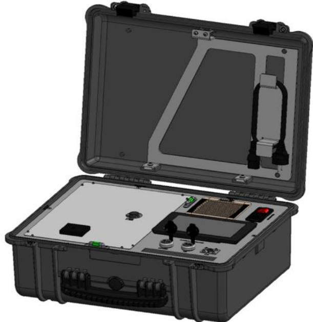
Both sensors have the same structural design, same batteries, Raspberry and touchscreen display, electrical connections and plugs. Only sensing devices and light sources (and their electronic control) are different.
