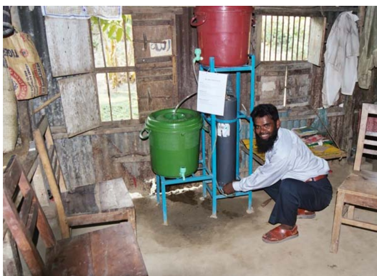
Figure 9. IHE arsenic removal filter in use in rural Bangladesh
