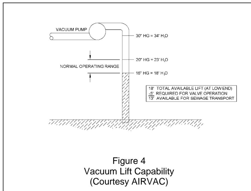
Static losses are those incurred by using lifts, or vertical profile changes. Profile changes are accomplished by using two 45-degree fittings joined by a section of pipe. For efficient use of the energy available, profile changes should be as small as possible. Numerous lifts are recommended over one large lift (AIRVAC, 2005). Table 3 shows the recommended lift height for various pipe sizes.
