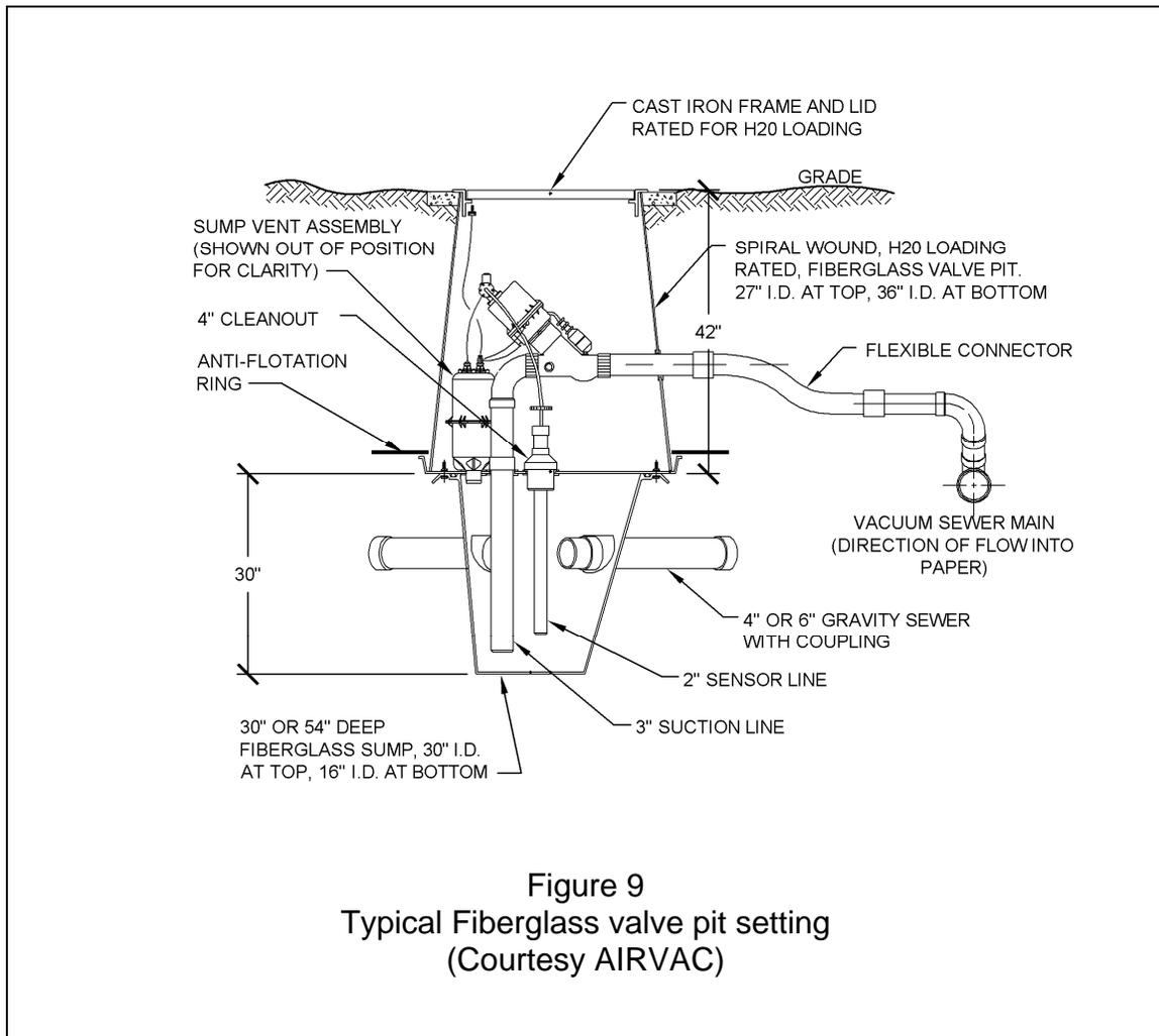
Up to four separate building sewers can be connected to one sump, each at 90 degrees to one another. However, this is rarely done as property lines considerations and other factors may render this impractical. By far, the most common valve pit sharing arrangement is for two adjacent houses to share a single valve pit (AIRVAC, 2005)
