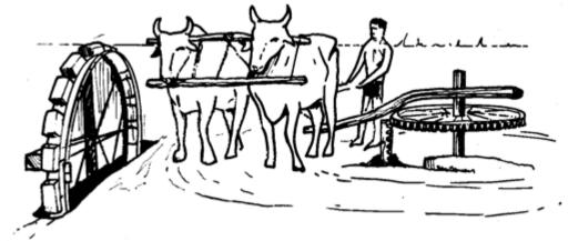
Figure 6: Animal Driven Persian Wheel Source: Water Pumping Devices
