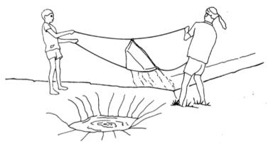
Figure 2: Swing Basket Irrigation Source: Water Pumping Devices
