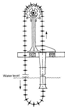
Figure 12: Chain and Washer Pump
