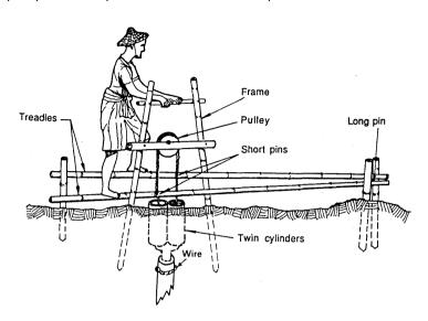
Figure 10: Treadle Pump
