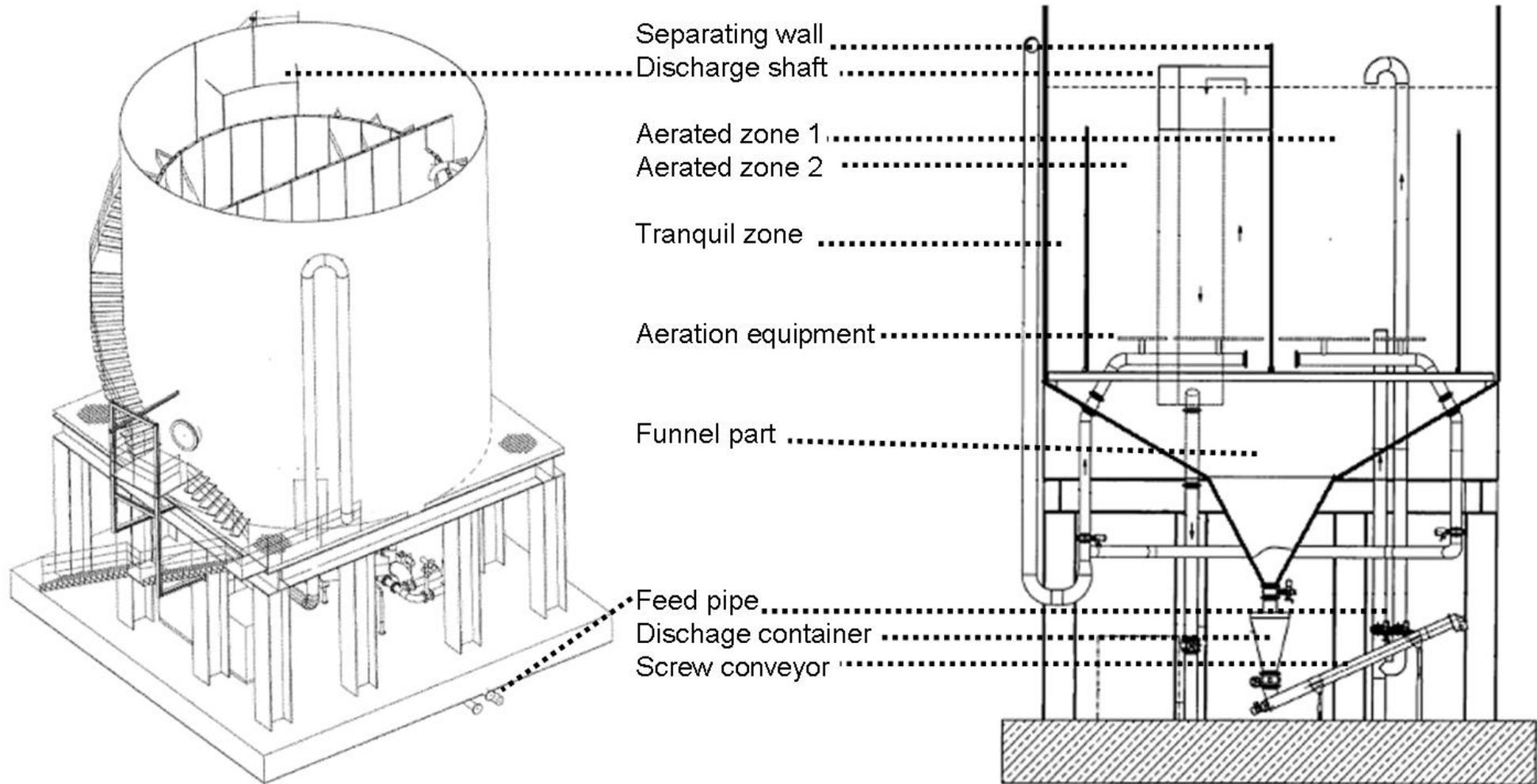
Figure 28: The AirPrex Reactor from above (Lengemann 2010a) and side (Hannemann *et al.* 2009).
