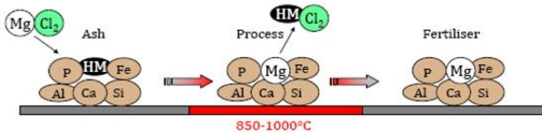
**Figure 21: Thermo-chemical process principle (Hermann 2009b)**
