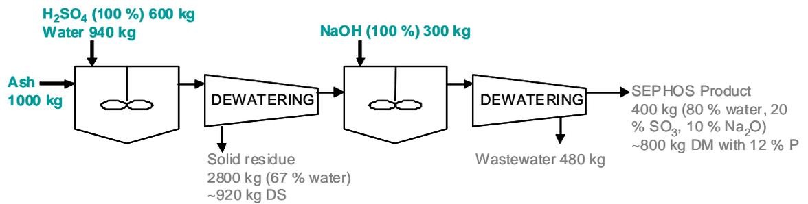
**Figure 43: Mass flow in the SEPHOS Process (modified from Schaum 2007).**
