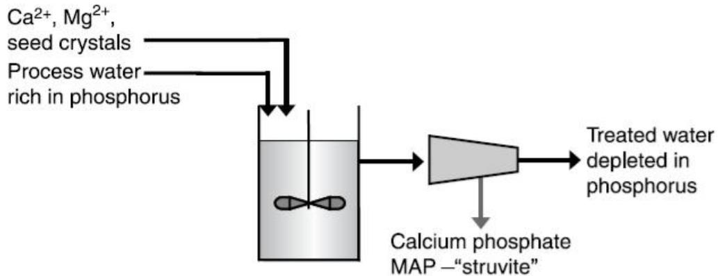
**Figure 18: Principle of crystallization and precipitation process (Cornel and Schaum 2009).**
