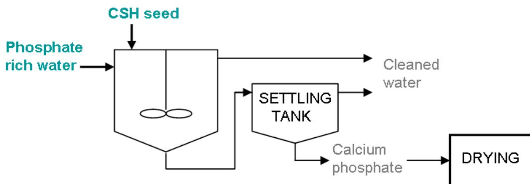
Figure 38: The P-RoC process flow chart (Berg and Schaum 2005).
