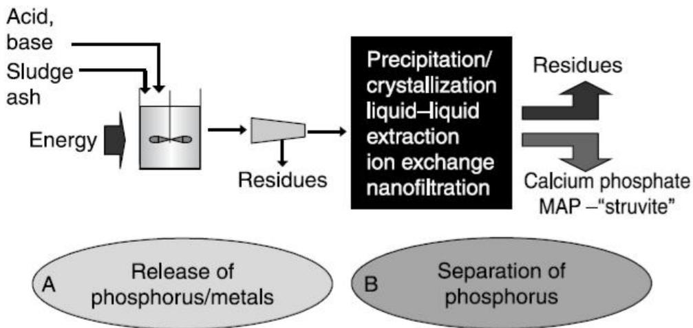
**Figure 19: Principle of wet chemical process (Cornel and Schaum 2009).**
