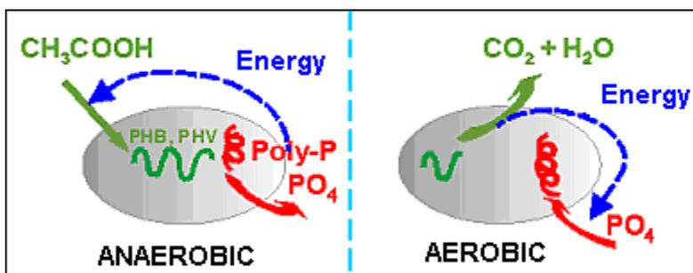
Figure 9: The principle of the cell operations for biological phosphorus removal (SYKE 2010).
