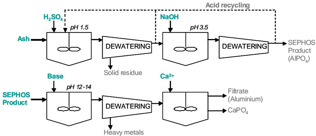
**Figure 42: The SEPHOS Process and the Advanced SEPHOS Process (modified from Schaum *et al.* 2005).**
