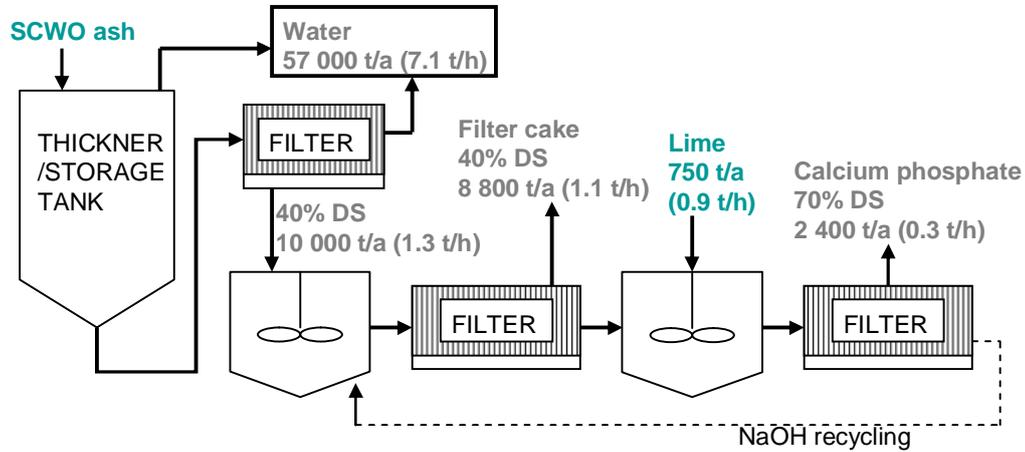
**Figure 46: The recycling step after SCWO in the Aqua Reci process (Stendahl and Jäferström 2004).**
