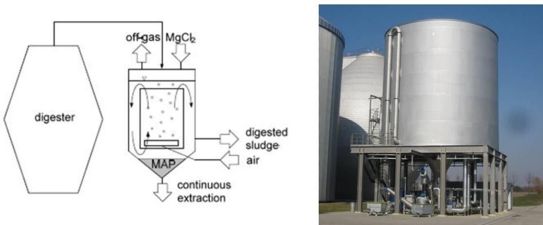
Figure 26: The AirPrex procedure (Heinzmann 2009) and reactor (Picture: J. Nieminen).
