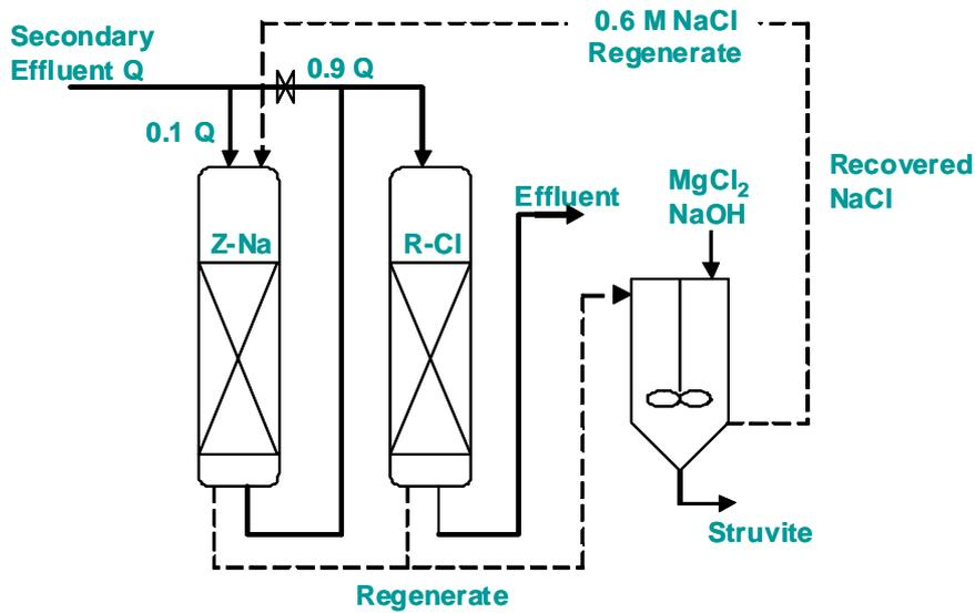
Figure 41: The “P-driven” Rem Nut® ion exchanger process flowchart (Liberti *et al.* 2001).
