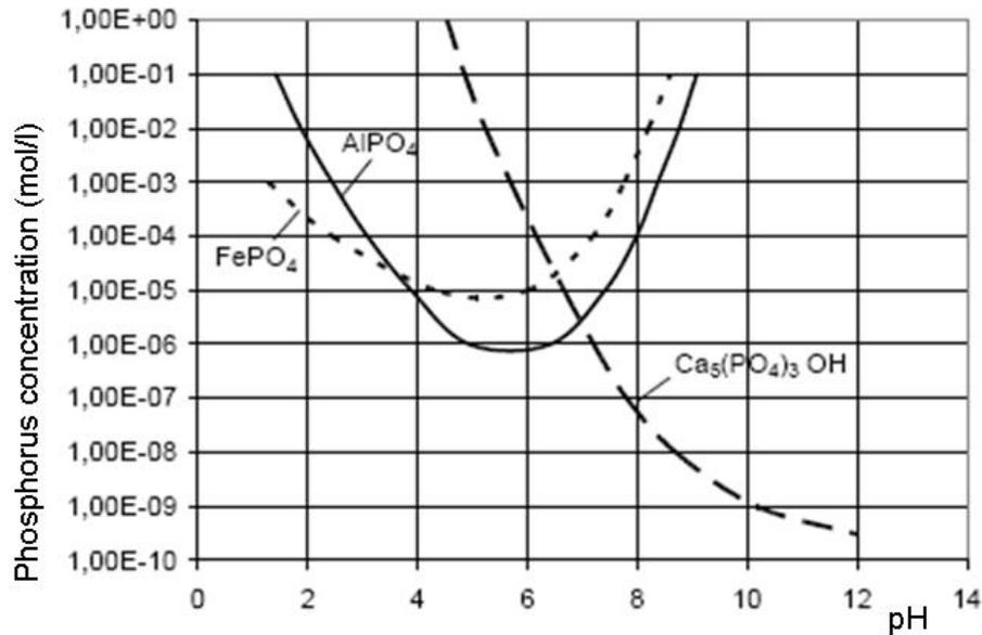
**Figure 8: The phosphate precipitants and pH (Montag 2008).**
