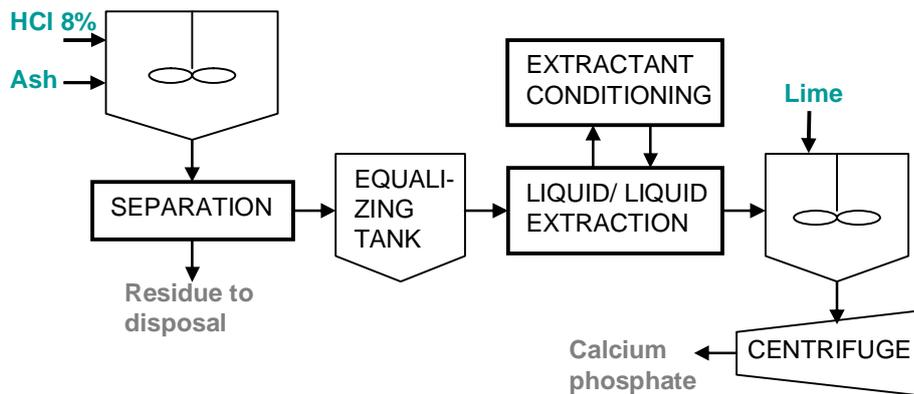
**Figure 44: The PASH process flow chart (modified from Montag 2009).**
