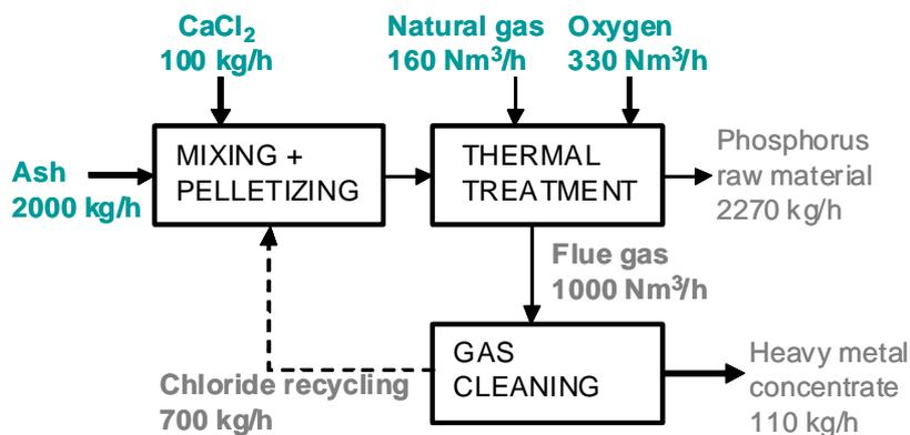
**Figure 48: The ASH DEC Process and estimated material flow of a full-scale plant with feed of 2000 kg/h of ash (ASH DEC 2010).**
