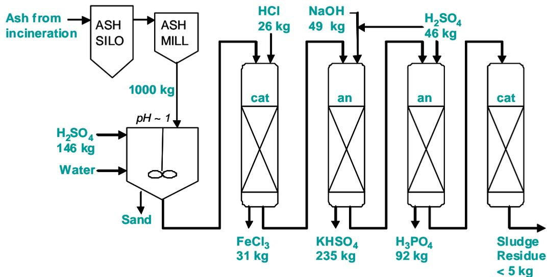
**Figure 45: The recovery unit of BioCon® Process with mass flow information from the pilot plant at Brønderslev WWTP (modified from Levlin 2002 and Hultman *et al.* 2001).**
