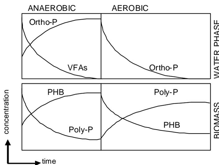
**Figure 10:** The concentrations of  $\text{PO}_4\text{-P}$ , VFA, PHB and polyphosphates in aerobic and anaerobic stage in water phase and in biomass (Janssen *et al.* 2002).
