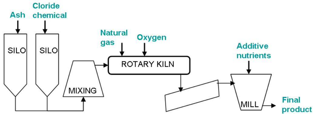
**Figure 47: The flowchart of the ASH DEC Process (modified from ASH DEC 2010).**
