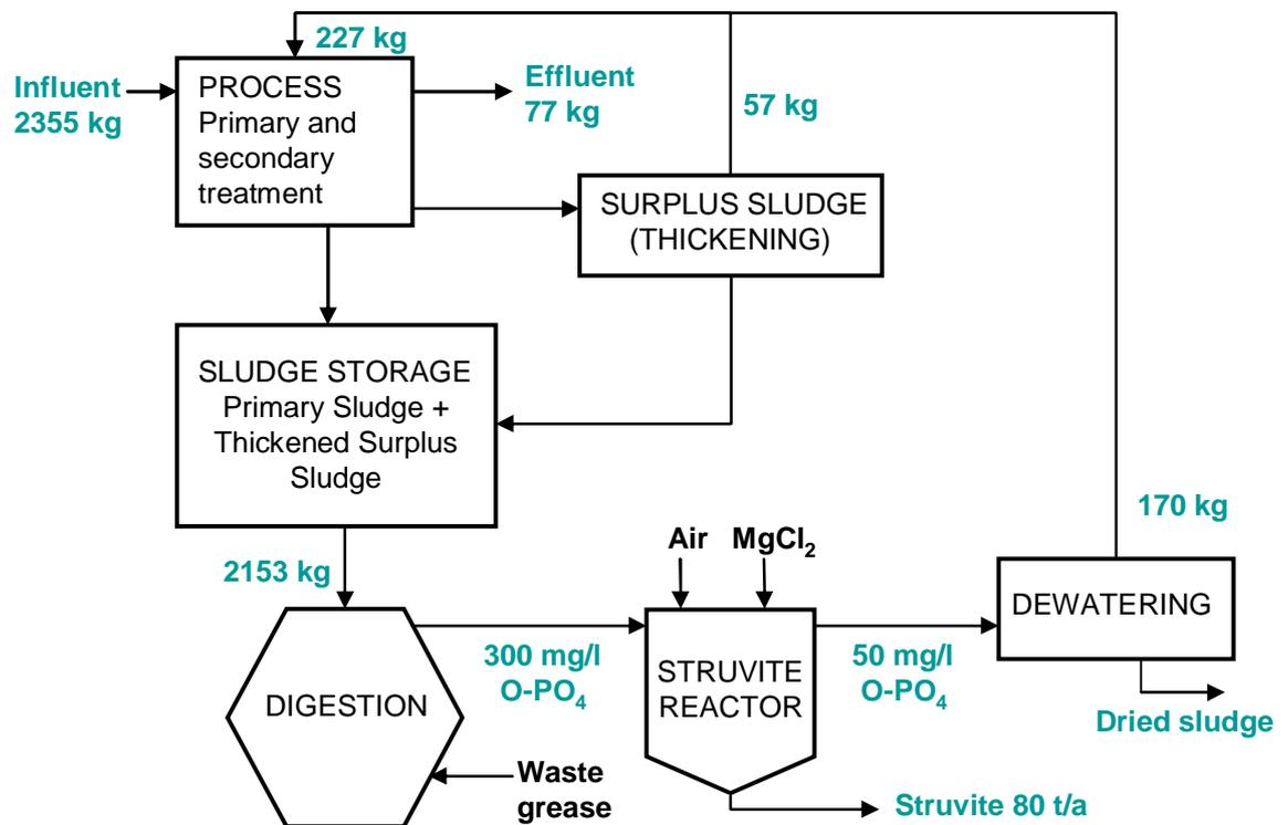
Figure 25: The daily phosphorus balance (kg/d) at WWTP Waßmannsdorf with the “old method” (modified from Lengemann 2010a).
