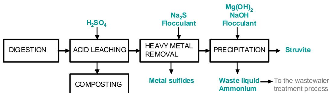
Figure 36: Flowchart of the Seaborne process at Gifhorn (Bayerle 2010).
