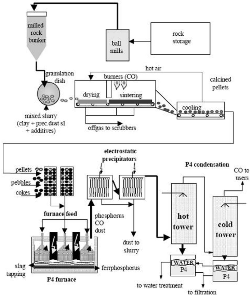
Figure 7: Electro-thermal production of elemental phosphorus (Schipper *et al.* 2001).
