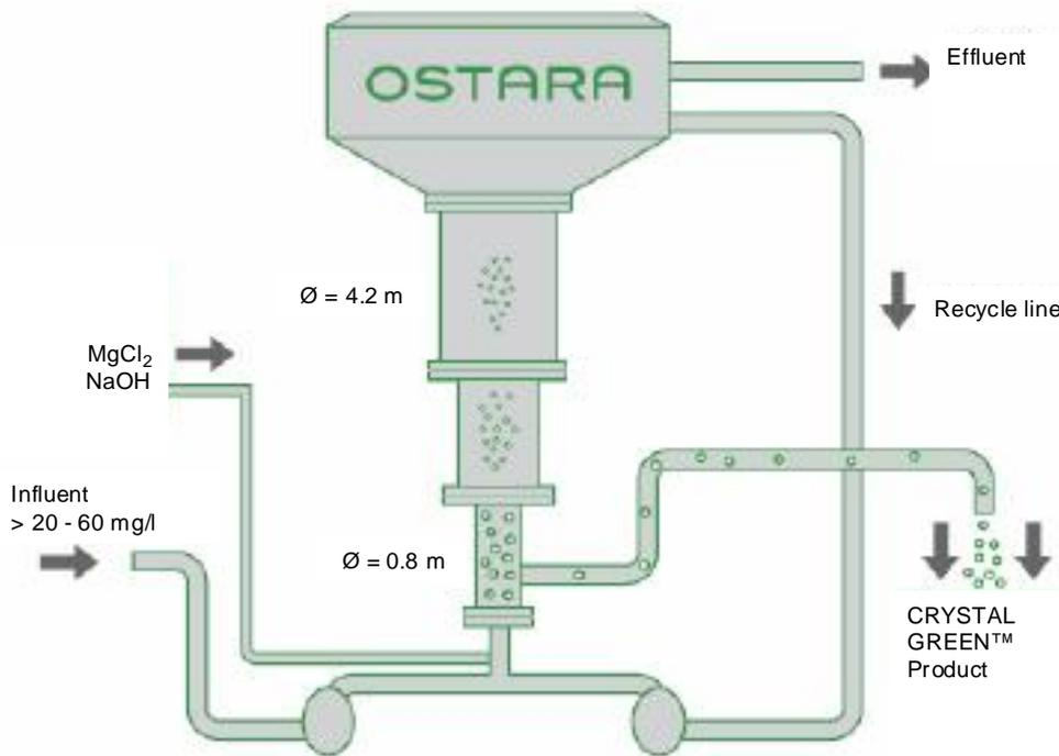
**Figure 31: The Ostara struvite precipitation reactor Pearl® (modified from Ostara 2010).**
