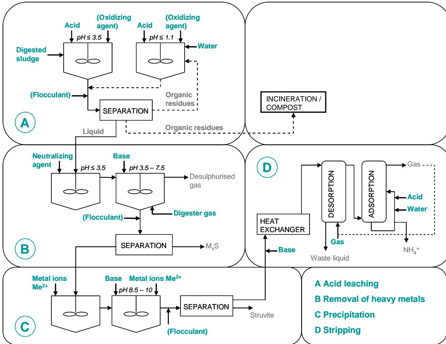
Figure 35: The patented version of the Seaborne process (modified from Vesterager 2009).
