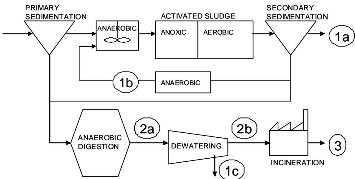
**Figure 13: Possible locations for phosphorus recovery (modified from Adam 2009 and Cornel and Schaum 2009).**
