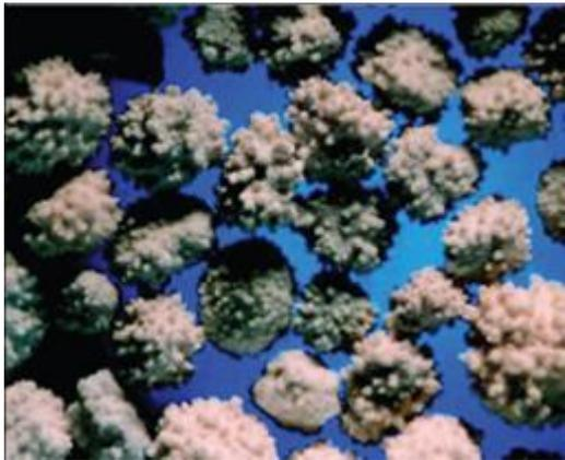
Figure 14: Calcium phosphate pellets (Giesen 2009a).
