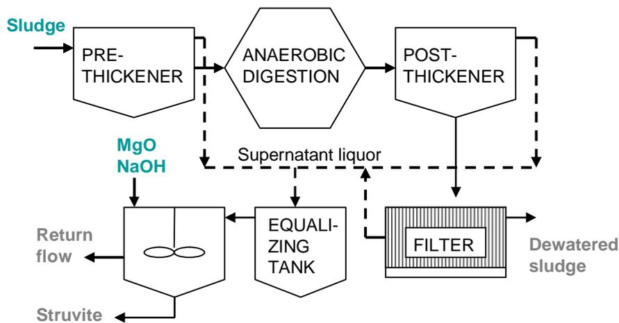
**Figure 40: Simplified flow chart of the PRISA process (Montag *et al.* 2007).**
