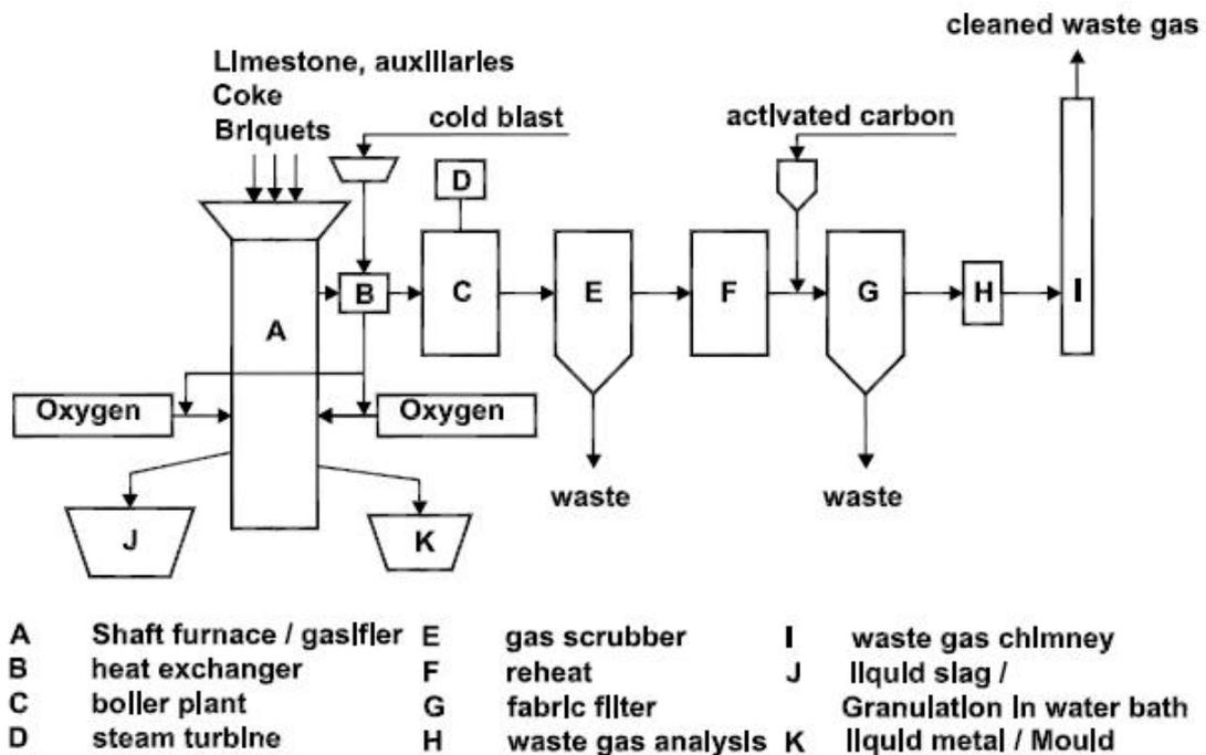
Figure 49: The Mephrec process (modified from Ignitec 2010).
