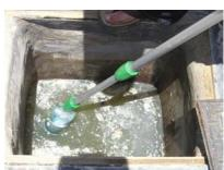
**Picture 9:** Sampling effluent from dome outlet (24.11.2008).
