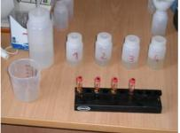
**Picture 11:** Hach Lange test cubes in the front (COD TNT822 and TNT823 were used).
