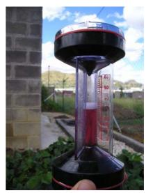
**Picture 21:** Testoryt device to measure the  $CO_2$ -content of gas.  $CO_2$  gets absorbed by the liquid. Thus the volume of the liquid increases correspondingly.
