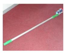
**Picture 1:** Effluent sampling stick. This sticks enables to samples through the tight cover holes of the ABR.
