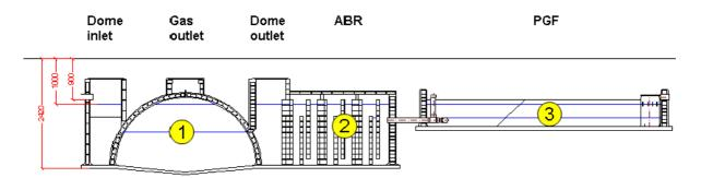
**Figure 2:** Scheme of DEWATS-Biogas-System of TED-Borda. The basic buildup consists of a digester (1), an anaerobic baffled reactor (ABR,2) and an planted gravel filter (PGF,3).
