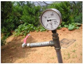
**Picture 2:** Gas tightness is first controlled in the gas piping system that goes from the digester outlet to the end users (for example stove).
