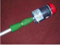
**Picture 2:** A bottle is cut into half and attached to stick.
