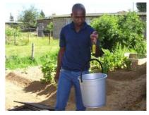
**Picture 24:** The feedstock material is weighed with a hanging balance before put into the inlet chamber.
