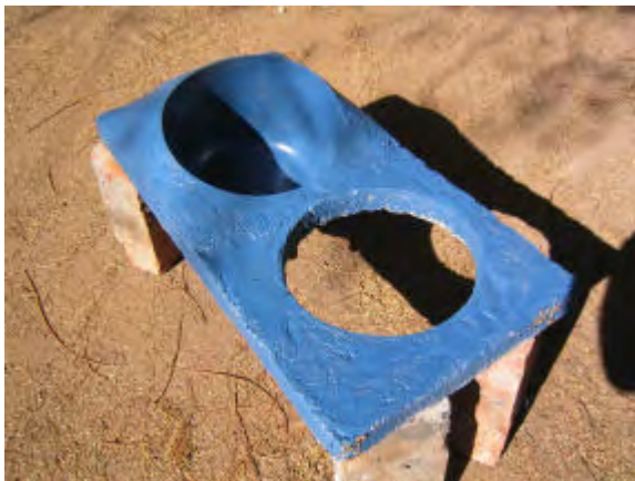
Hand made examples of urine diverting devises. On the left, a urine diverting squat plate and on the right a urine diverting pedestal. Both use plastic buckets as part of the construction.
