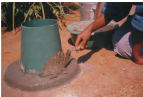
Very low cost pedestal made from a ten litre plastic bucket and cement only. It is durable and with suitable painting can be made very smart.
