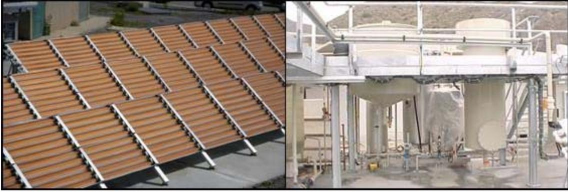
**Figure 1.** Views of the combined solar photo-Fenton /biological demonstration plant. Solar collector field (left), conditioner tank and Immobilised Biomass Reactor (right).
