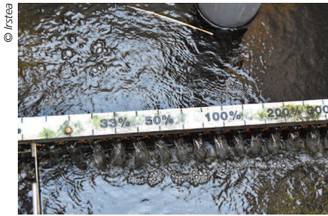
Figure 6. V-notch weir plate for manual recirculation.
