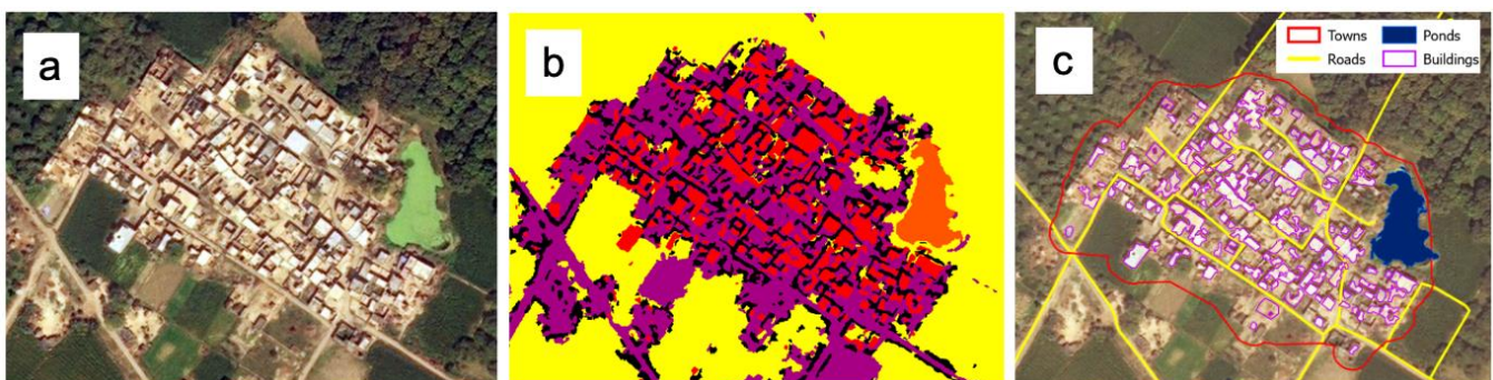
Figure 3. Image classification process: (a) raw satellite image, (b) image classification process, and (c) conversion to feature and extraction of the data. Delineation of roads was completed manually and processed so the feature data could later be used for the network analysis tool.
