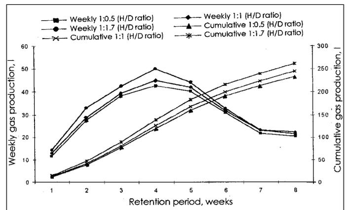
Figure 4 Weekly and cumulative gas production from donkey-dung alone (control) in three different size (H/D ratio) digesters
