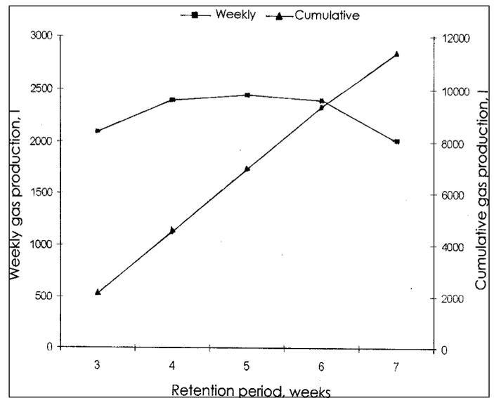
Figure 5 Weekly and cumulative gas production from poultry droppings and donkey-dung combination in pilot size biogas plant
