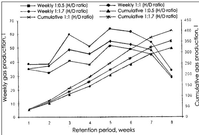
Figure 1 Weekly and cumulative gas production from poultry droppings and donkey-dung combination in three different size (H/D ratio) digesters
