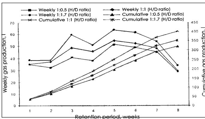
Figure 2 Weekly and cumulative gas production from parthenium and donkey-dung combination in three different size (H/D ratio) digesters
