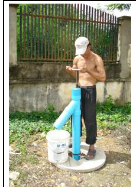
Figure 1 - The Gulper – a handpump for emptying latrine pits
