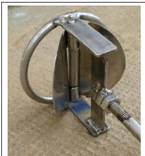
Figure 2- Inner valve on the bottom of the puller rod
