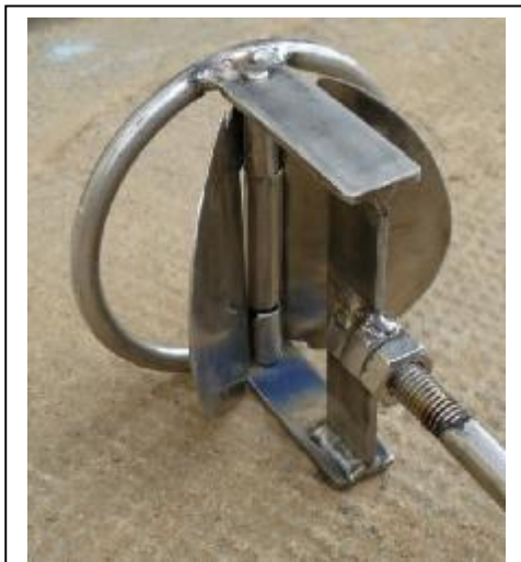
Figure 2- Inner valve on the bottom of the puller rod
