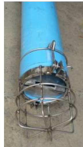
Figure 3 - Strainer and valve at the bottom of the riser pipe
