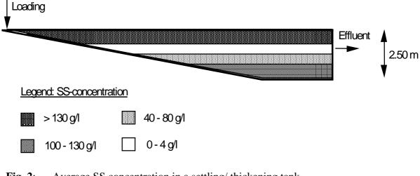
**Fig. 2**: Average SS concentration in a settling/ thickening tank after 4 weeks of operation and 1 week at rest (Achimota FSTP, Accra).
