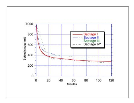
**Fig. 1**: Results of settling tests performed in 1-litre cylinders (septage I-III) and in a cylinder of 20 cm diameter and 2 m height (septage IV\*)
