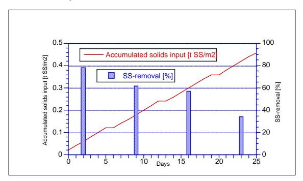
**Fig. 3**: Accumulated Solids Loading and Removal Efficiency in the Sedimentation/Thickening Tank as a Function of the Loading Duration
