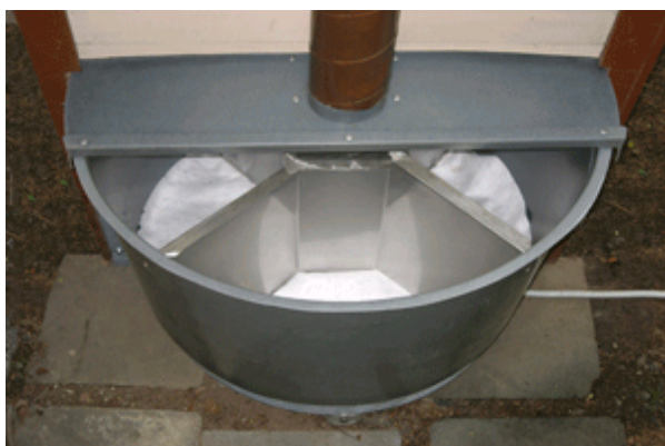
Figure 10. Rotating multi-chamber bin (source: Ekolet, Finland).
