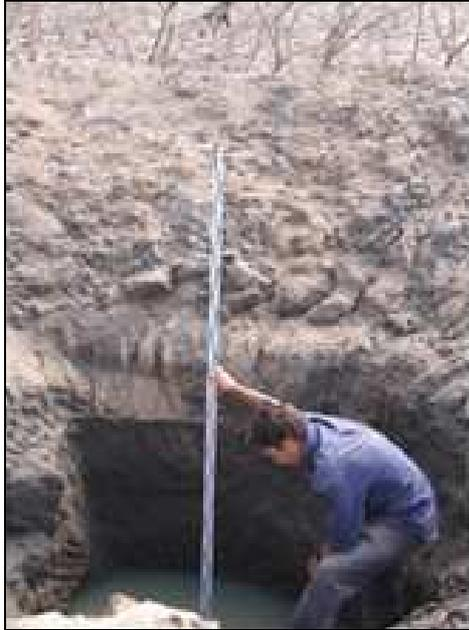
**Figure 2-6:** Silt layer under the sandy layer behind a sand storage dam
