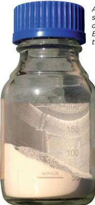
A sample of struvite produced in the Eawag laboratory.
