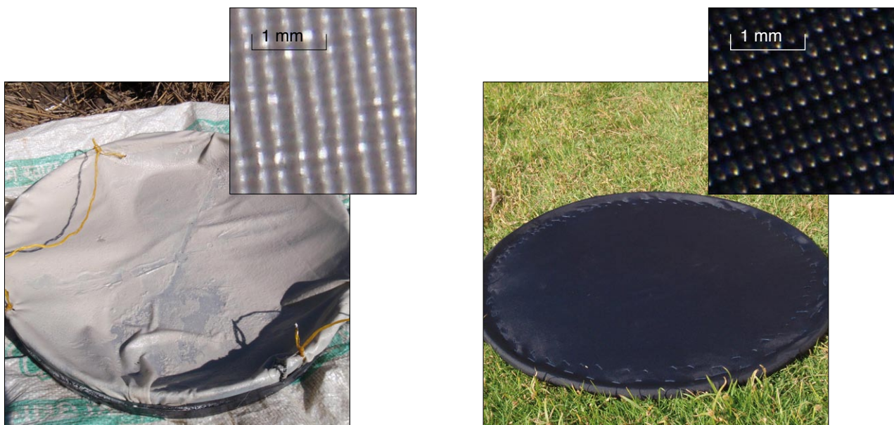
Figure 7: The 2 tested filter arrays in the first STUN reactor. Left: cotton fabric ( d_{\text{pore}} < 200 \mu\text{m} ) on a welded steel and wire mesh assembly. Right: nylon fabric ( d_{\text{pore}} < 100 \mu\text{m} ) sewn to an iron ring.
