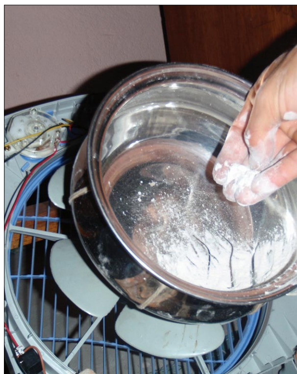
Figure 19: Experimental rotating steel drum for struvite granulation constructed from a fan motor and steel pot (20 cm diameter).
