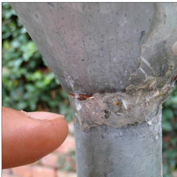
Figure 13: Detail on the reactor tank assembly: lower outlet reinforcement through soldering and crimped and riveted seam along the reactor side.
