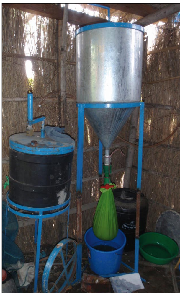
Figure 15: Overall view of the improved pilot scale struvite recovery reactor (right), beside the first reactor (left).
