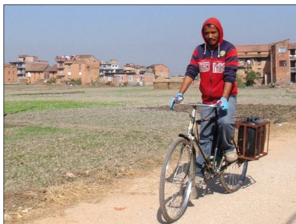
Figure 4: The 'pee-cycle' used to collect urine from a dozen households in the field study site's neighbourhood.
