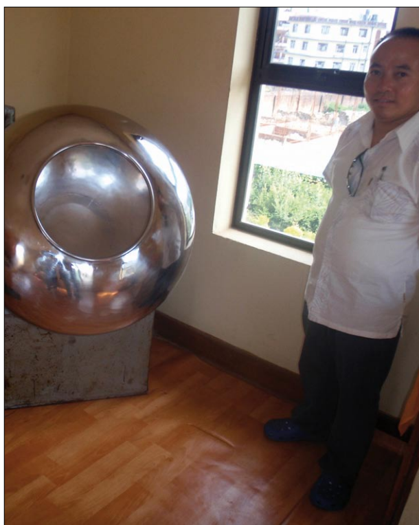
Figure 18: Production of granules from medicinal powder as practiced in Tibetan medicine by means of a revolving steel drum (Shechen Clinic, Kathmandu).
