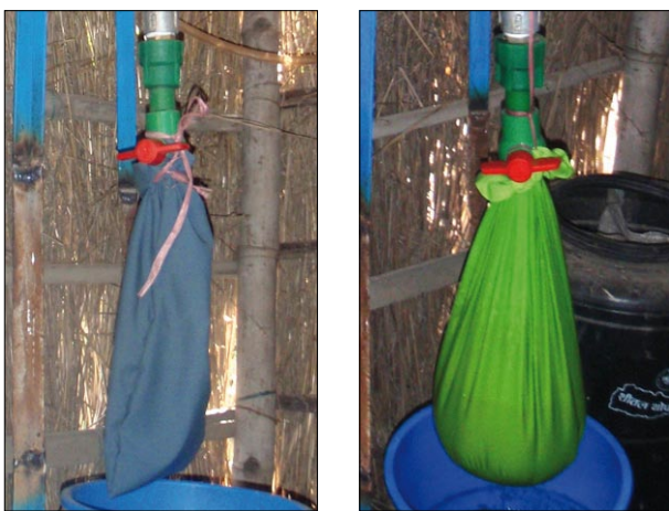
Figure 12: Two filter bags tested for their performance: Left: Rectangular shape with approximately 1500 \text{ cm}^2 filtering surface; Right: Cylindrical shape with approximately 2000 \text{ cm}^2 filtering surface.
