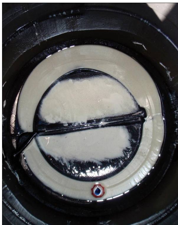
Figure 6: Struvite powder sedimented at the reactor's bottom, due to low filter efficiency.
