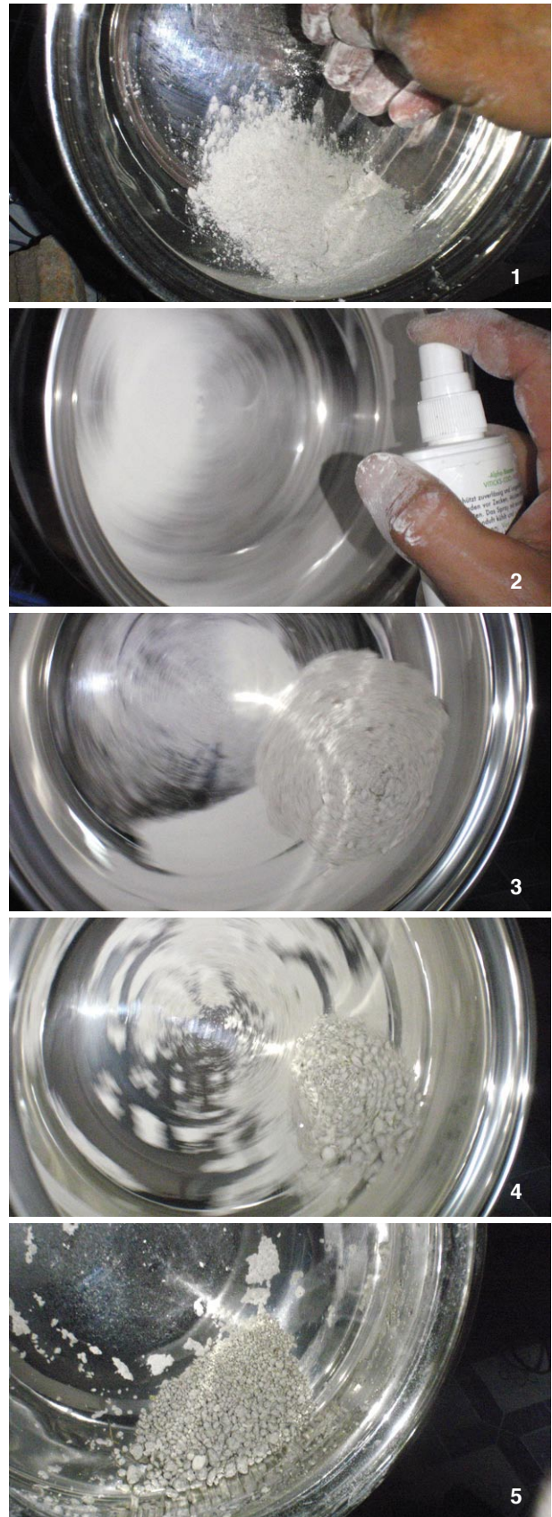
Figure 34: Production of granules from struvite powder: 1. Powder being added to the rotating drum, 2. Addition of water by means of a vaporizer, 3. Formation of low diameter granules, 4. Increase in granule diameter after few minutes, 5. The finished granules in the drum.
