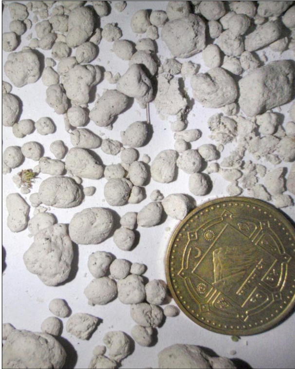
Figure 33: The dried struvite granules (diameter of the 1-rupee coin: 20 mm).
