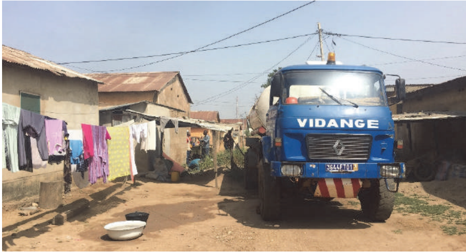
Figure 1.2.2. A truck desludging a household pit latrine.
