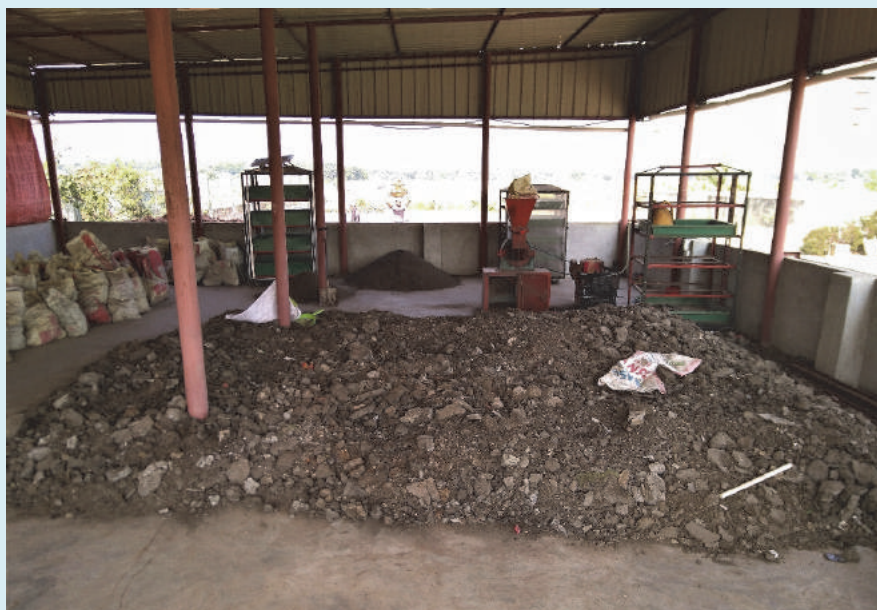
Figure 2.3.5 Preparation of the dewatered sludge cakes in Faridpur, Bangladesh, prior to transportation to the nearby co-composting plant.
