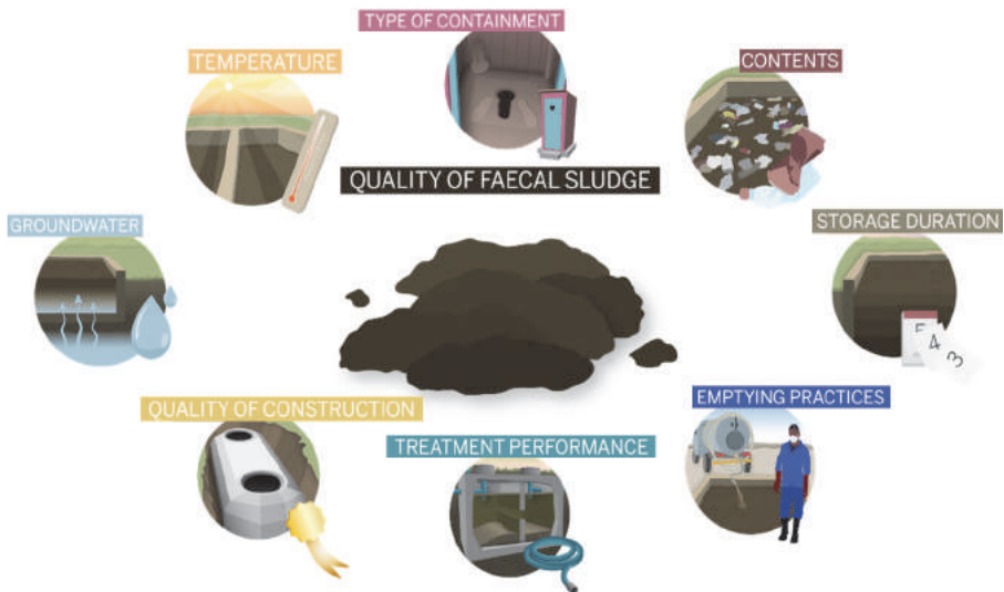
Figure 1.1.3 Parameters that can affect faecal sludge characteristics. Taken from the MOOC Introduction to Faecal Sludge Management .
