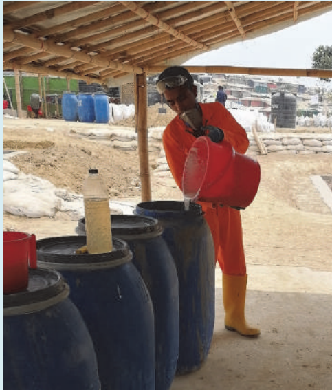
Figure 5.5.2 Operator pouring the lime slurry into a barrel filled with faecal sludge in Cox's Bazar, Bangladesh.
