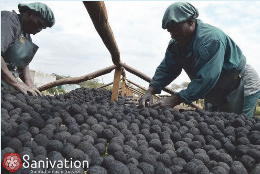
Figure 5.3.3 Workers at the Sanivation plant in Naivasha putting the briquettes on drying racks to dry (photo: Sanivation).
