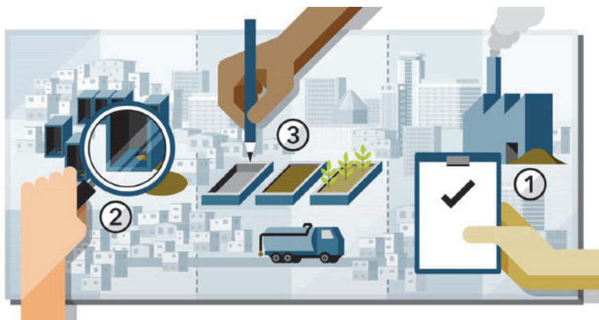
Figure 1.2.1 The engineering design approach to faecal sludge management: (1) first, treatment objectives and performance goals are set; (2) then quantities and qualities (Q&Q) of incoming faecal sludge are estimated; and (3) finally a selection of treatment technologies or management solutions is evaluated. Figure supplied from Strande et al. , (2016).
