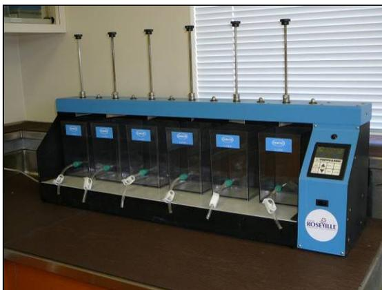
**Wagner™ Jar – p/n 41170-00, 2-liter square plastic flocc jar for the jar test. The Wagner Jar has a tap near the bottom of the jar to facilitate withdrawal of a sample for further testing of pH, turbidity, alkalinity, streaming current, zeta potential, etc. Photo by author.**
