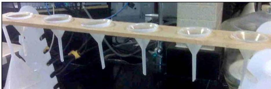
**Figure 21: Six-place assembly for filtering samples after a jar test.
