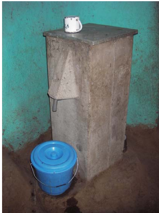
Figure 2.2.1: BioSand Filter in Koftu village, Oromia region, Ethiopia
