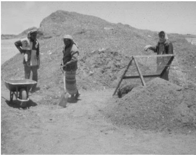
Photo 7. Inclined manual screen in use in Dhamar, Yemen Photo: ©WASTE, Arnold van de Klundert
