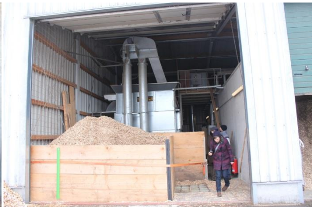
Figure 50: Feed-and-turn drier for woodchips installed at a biogas plant in Germany (Source: Rutz D.).
