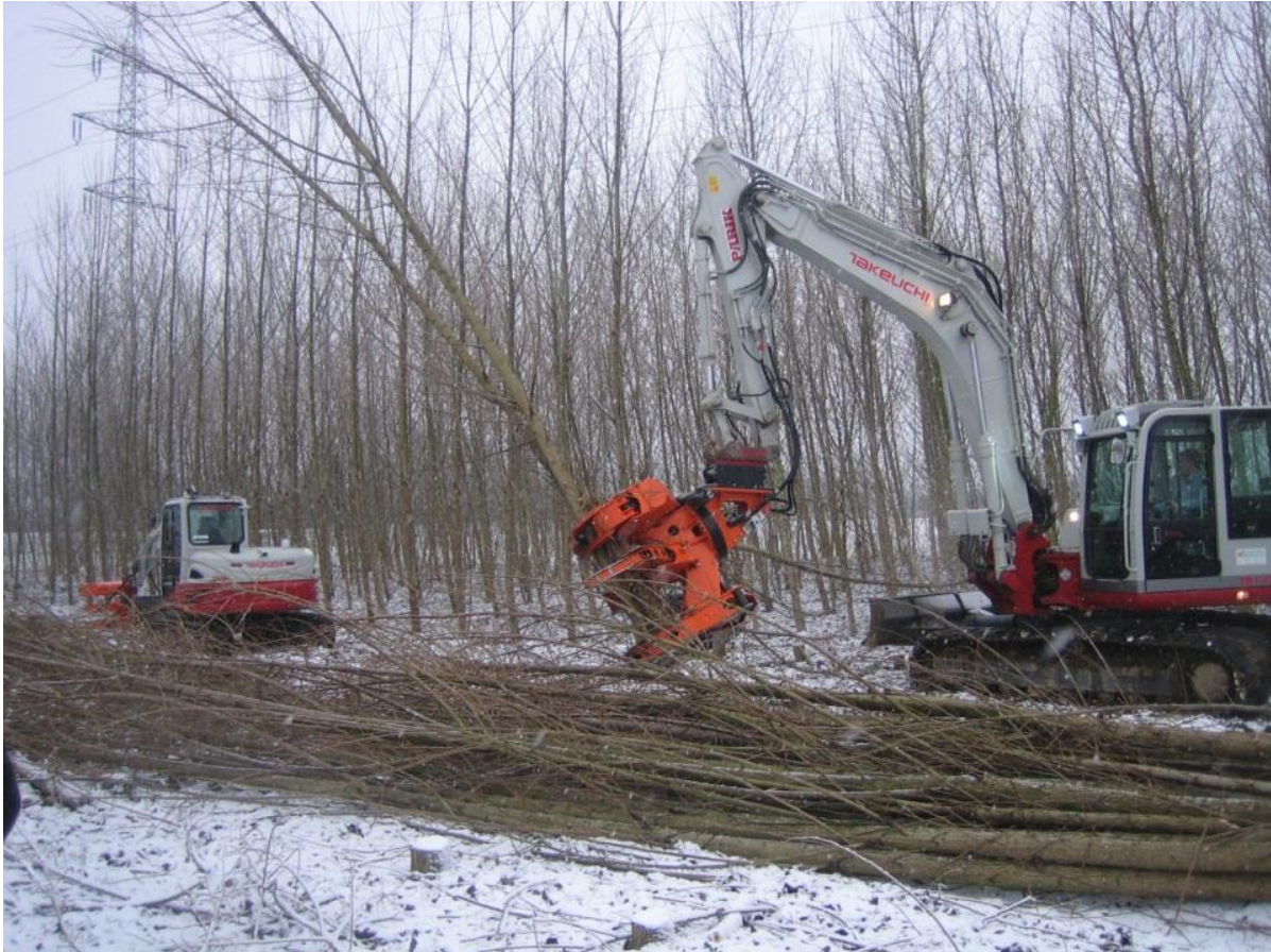
Figure 40: Gripper-head mounted on an excavator for harvesting poplar in Austria (Source: Mergner R.)
