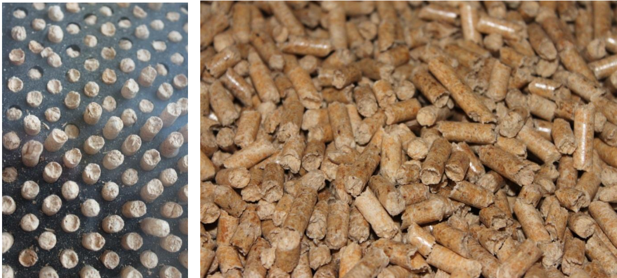
Figure 60: Pellet press (left) and high-quality pellets (right) (Source: Rutz D.)
