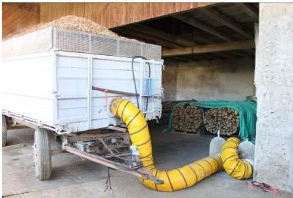
Figure 49: Charge dryer on a trailer using the waste heat of a biogas plant in Germany (Source: Rutz D.).
