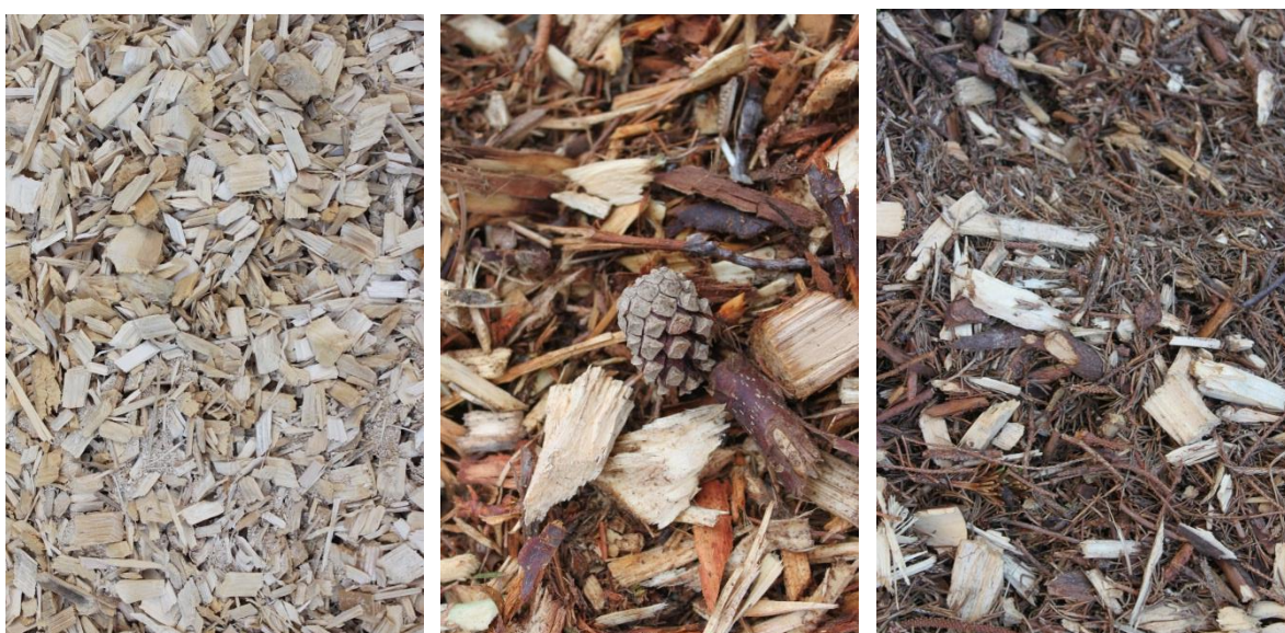
Figure 56: High quality (left) and low quality (middle, right) (non-SRC) woodchips in Germany (Source: Rutz D.)
