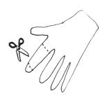
Cut the finger off of a disposable glove to make the top gasket.
