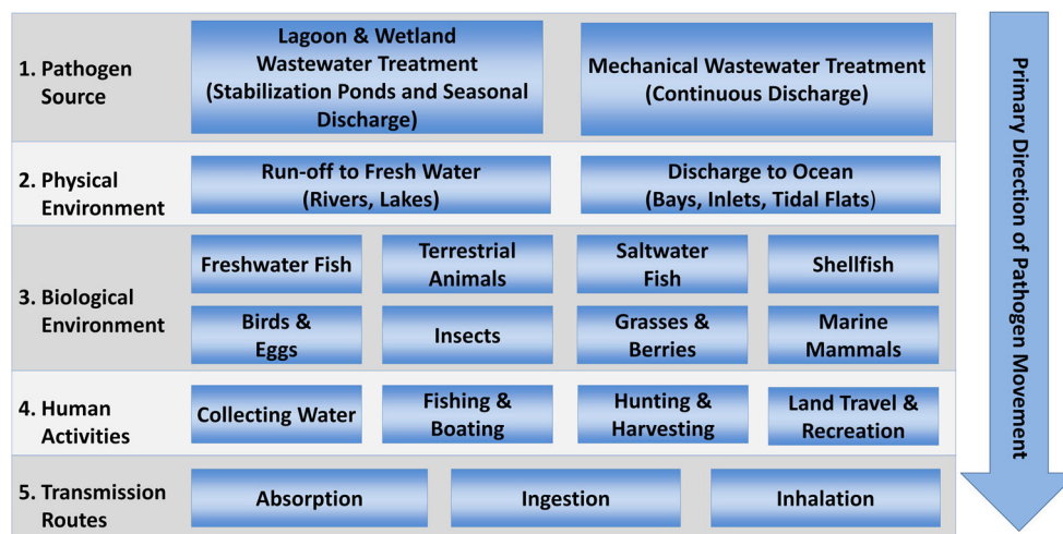
Fig. 1 A conceptual model of potential wastewater effluent exposure pathways in Arctic Canadian communities through five categories of factors
