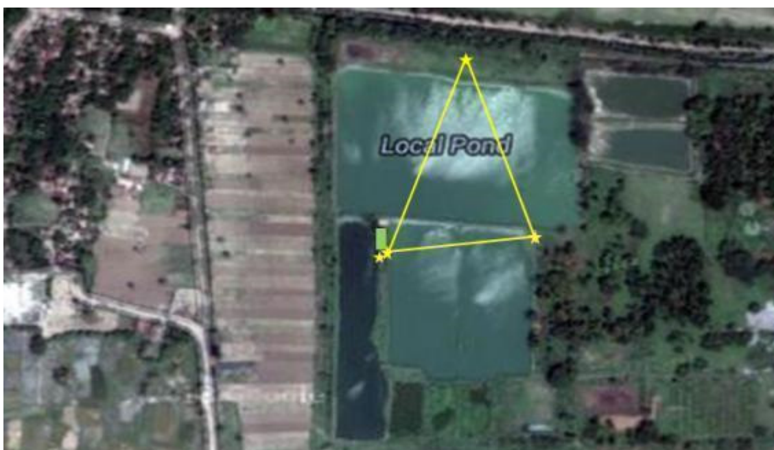
Figure 12: Top view of Kalyani STP Pond system (green square – disinfection system building; stars indicate the location of the BF wells and sampling wells forming the hydrological triangle).
