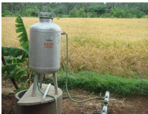
Figure20. Use of fertilisation tank for applying urine through drip irrigation (Photo: Prakash Kumar)
