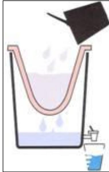
**Cross Section of Ceramic Pot Filter**
