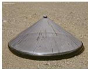
2. The evaporated Water condensates in the form of droplets on the inner wall of the cone. These droplets trickle down the inner wall into a circular trough at the inner base of the cone.
