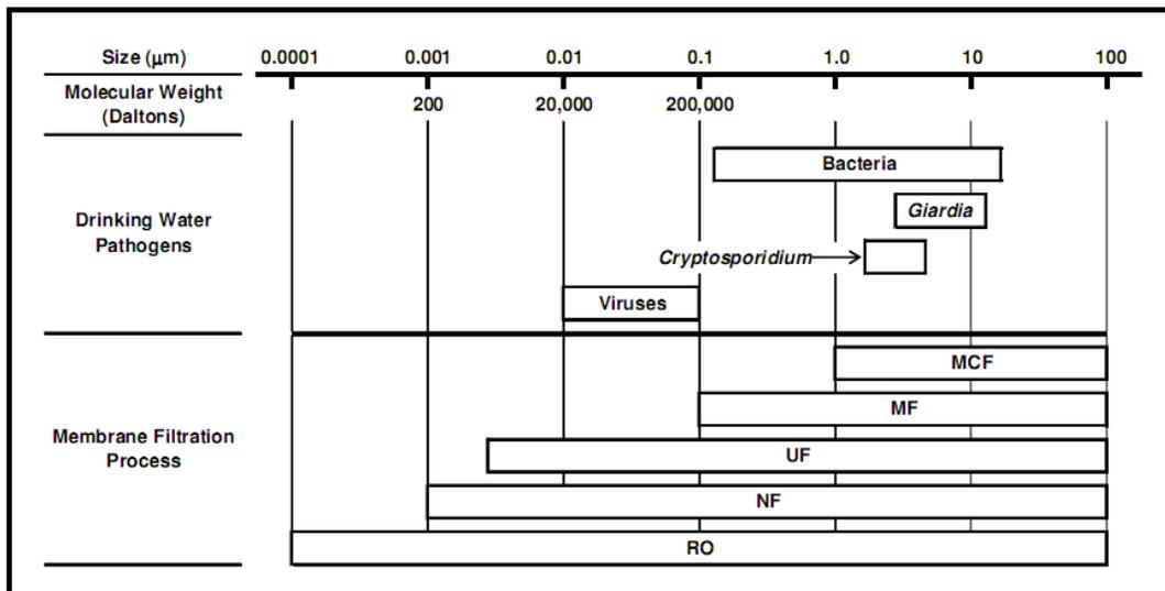
Pore Size for Various Filtration Types and Relative Pathogen Sizes ("MCF" = Membrane Cartridge Filtration)
