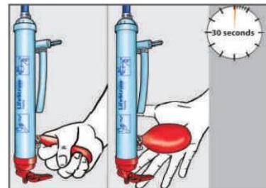
**Squeezing the bulb for backwash**
