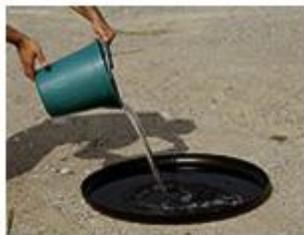
1. Pour salty / brackish Water into pan. Then float the WaterCone® on top. The black pan absorbs the sunlight and heats up the water to support evaporation..
