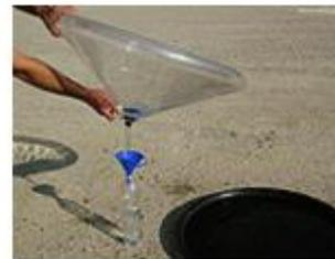
3. By unscrewing the cap at the tip of the cone and turning the cone upside down, one can empty the potable Water gathered in the trough directly into a drinking device.
