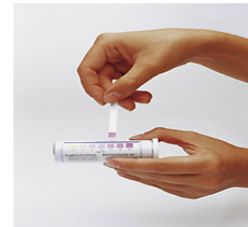
After the reaction time has passed, the colour of the reagent area is compared with the colour chart on the package to determine the concentration.
