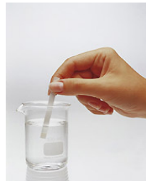
The reagent area is dipped into the water sample.
