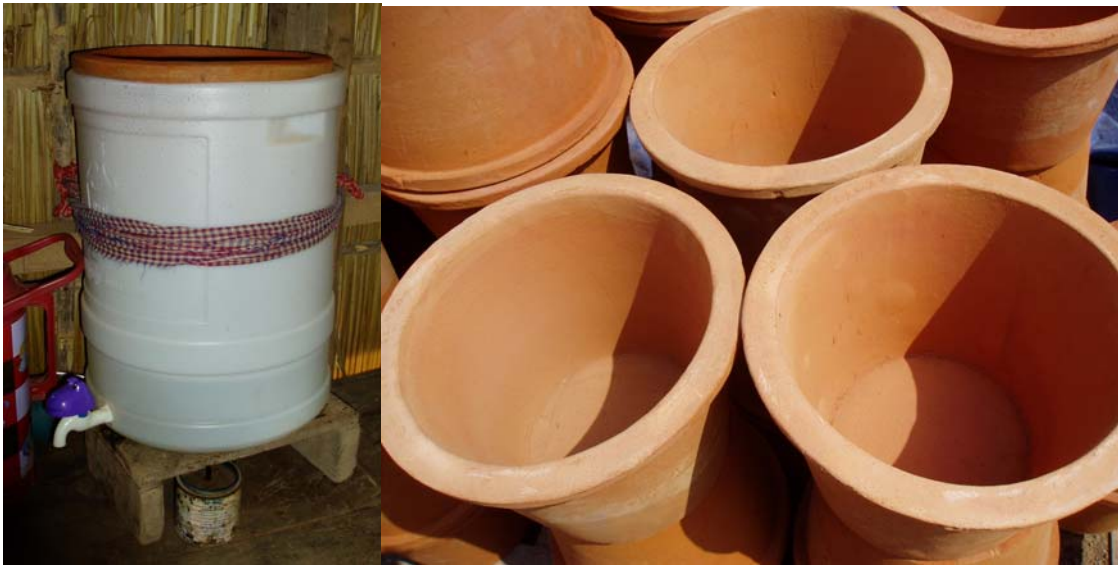
Figure 2.1. The ceramic water purifier (CWP) and porous ceramic pots stacked for drying, as manufactured by Resource Development International, Kandal Province, Cambodia. Porosity in the ceramic ( < 1 \mu\text{m} and larger) is created by mixing finely ground rice husks into the clay, which combust in the firing process to leave behind pore spaces. Water passes through the porous ceramic filter element by gravity (capacity approximately 10 l) at 1-3 l/hr into the receiving container (20 l), where it is dispensed via a tap to prevent post-filtration contamination of the product water through dipping or other contact with soiled hands or vessels. Filters are treated with a \text{AgNO}_3 solution to reduce microbial recontamination of the filter and biofilm formation and increase microbiological effectiveness.
