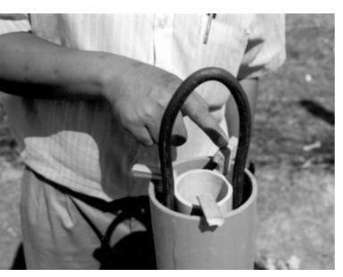
Figure 7.1 Construction of hollow weighted dummy – ready for filling for weight with cement
