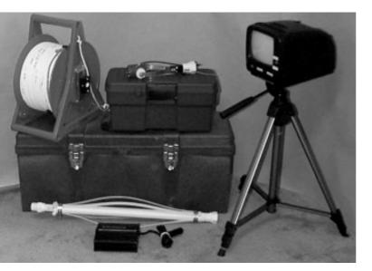
Figure 10.1 Borehole camera
