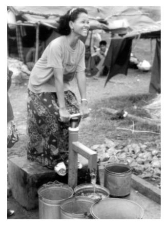
Figure 6.2 Direct Acting hand pump
