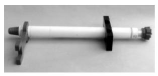
Figure 3.3 Down-the-hole hammer – with stripping clamp and spanner
