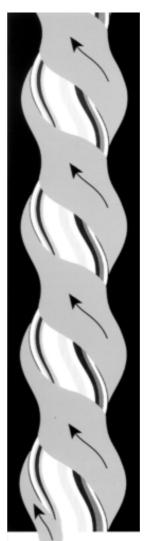
pumped fluid and the confining drill pipe. The capacity of the pump to remove material steadily from the bottom of the hole dictates the penetration speed of the drill bit.
