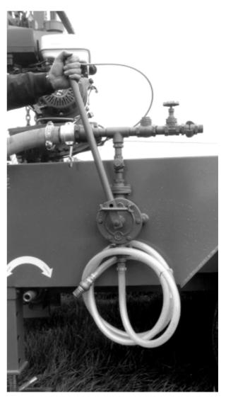
Figure 4.2 Semi rotary hand pump
