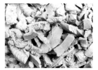
Figure 2.9 Individual clay cuttings washed to the surface
