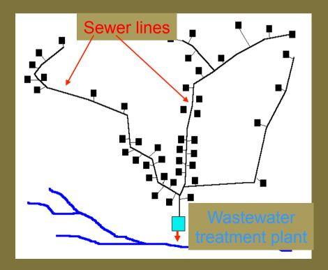
Initial investment costs for centralised sewage treatment systems make up for the largest part, i.e. 70 to 90% of the total cost of sewage treatment.
