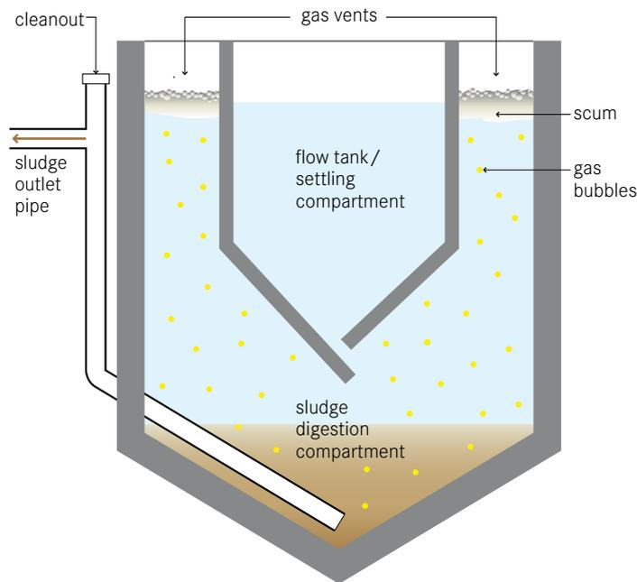
**The Imhoff tank is a primary treatment technology for raw wastewater, designed for solid-liquid separation and digestion of the settled sludge. It consists of a V-shaped settling compartment above a tapering sludge digestion chamber with gas vents.**
