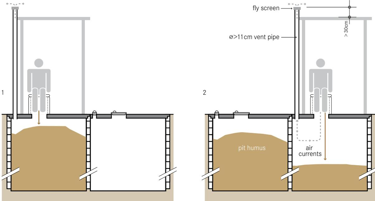
The double VIP has almost the same design as the Single VIP (S.3) with the added advantage of a second pit that allows it to be used continuously and permits safer and easier emptying.
