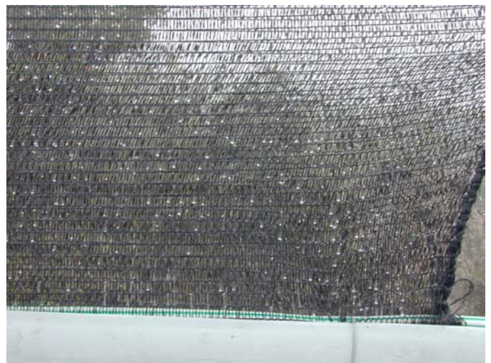
Figure 4: A double layer of a specially chosen polyethylene mesh is used to collect the fog droplets.
