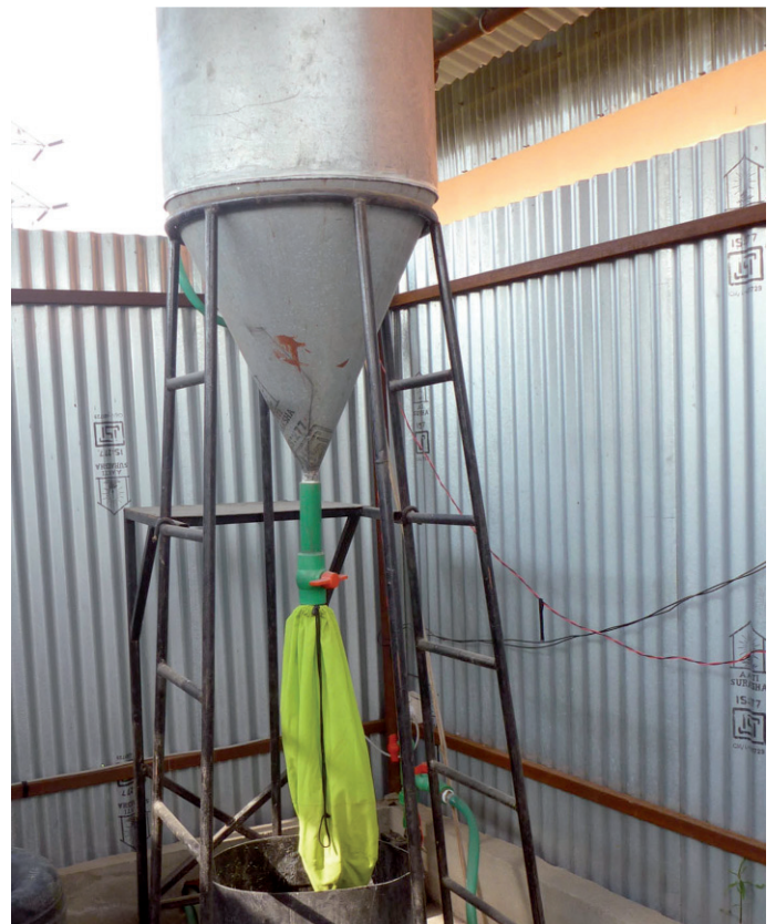
Figure 5: The struvite reactor with a nylon filter bag to separate the precipitated struvite powder from the liquid.
